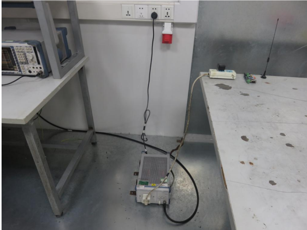
Photo of Power Line Conducted Emission Test
