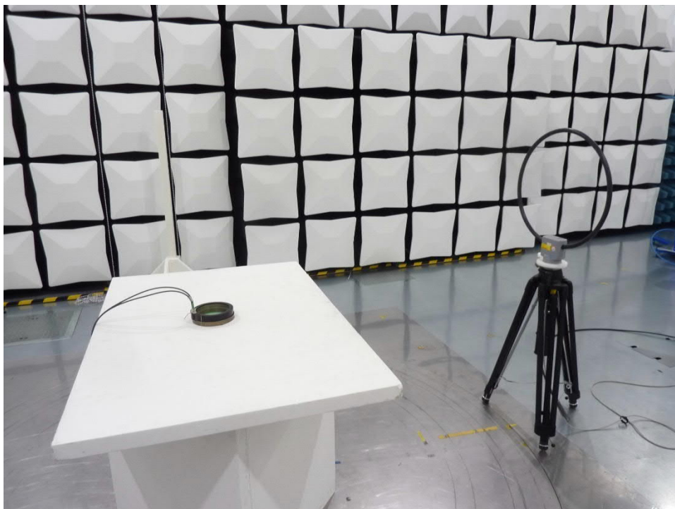
212050_02 Test setup 500 kHz to 30 MHz EUT in Z position
