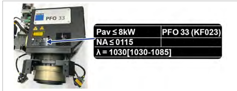
Specification on programmable focusing optics (example PFO 33)
