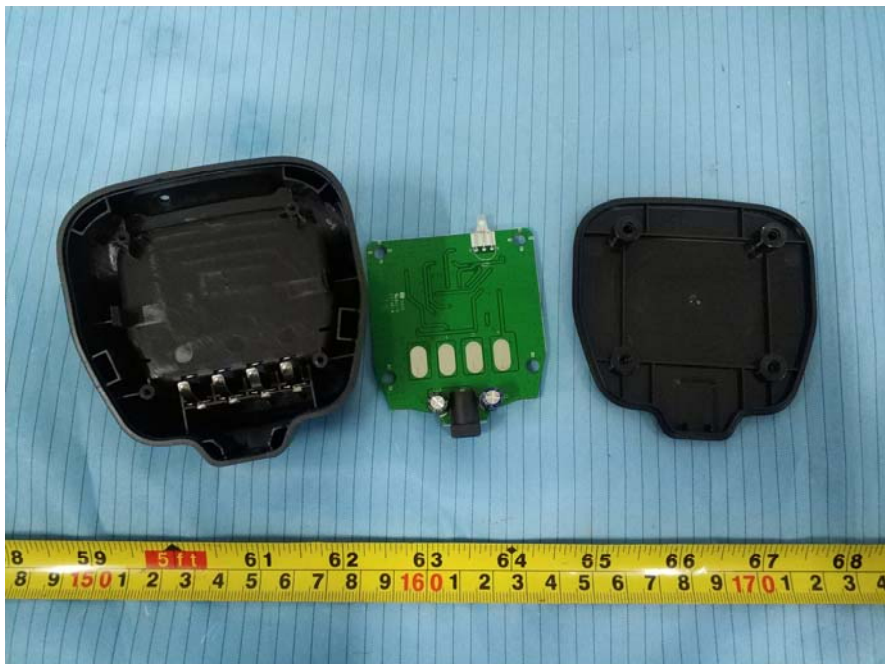
EUT (Charger) – Cover off View
