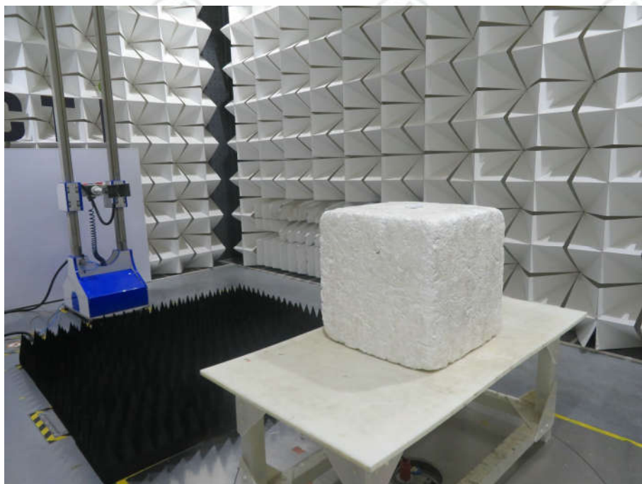
Radiated spurious emission Test Setup-3(Above 1GHz)
