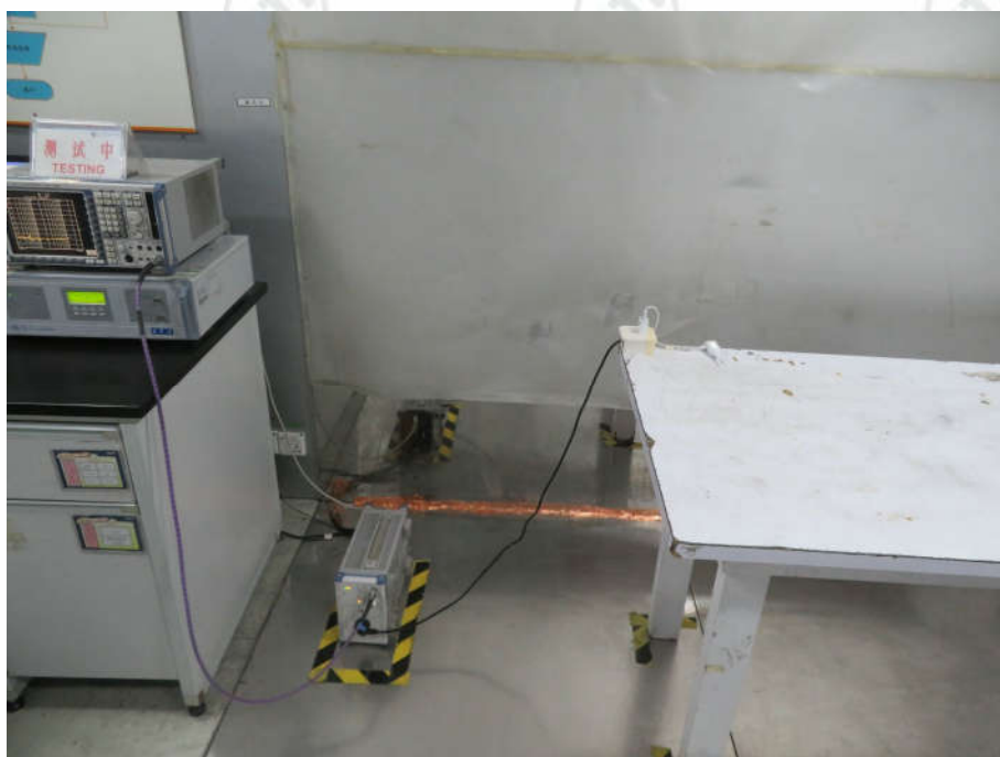
Conducted Emissions Test Setup
