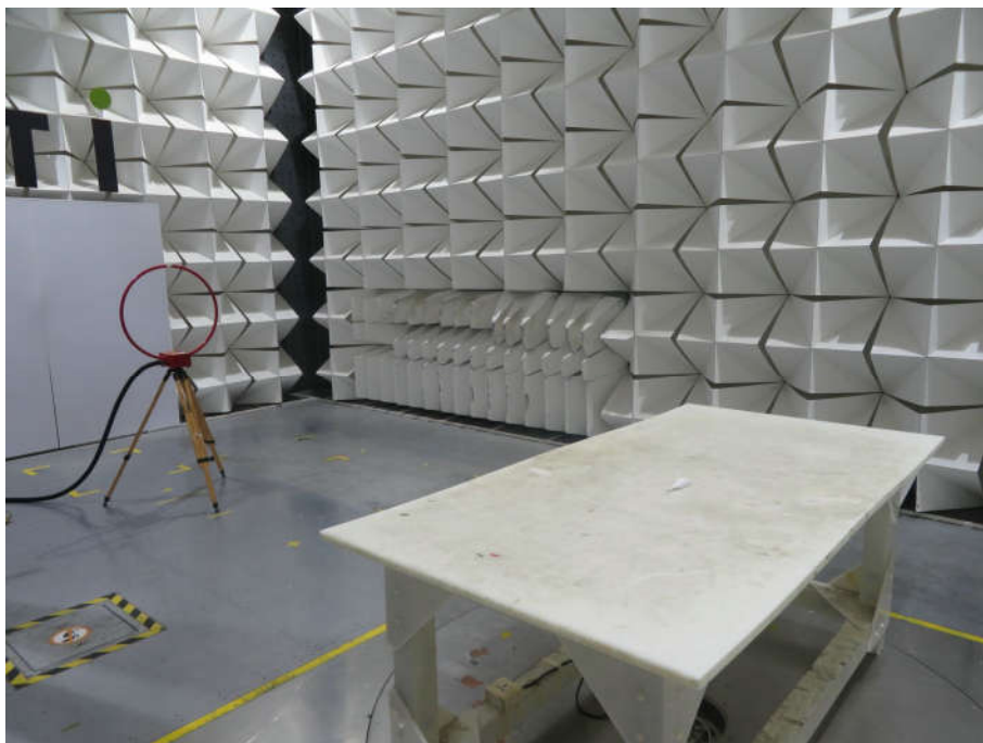
Radiated spurious emission Test Setup-1(Below 30MHz)
