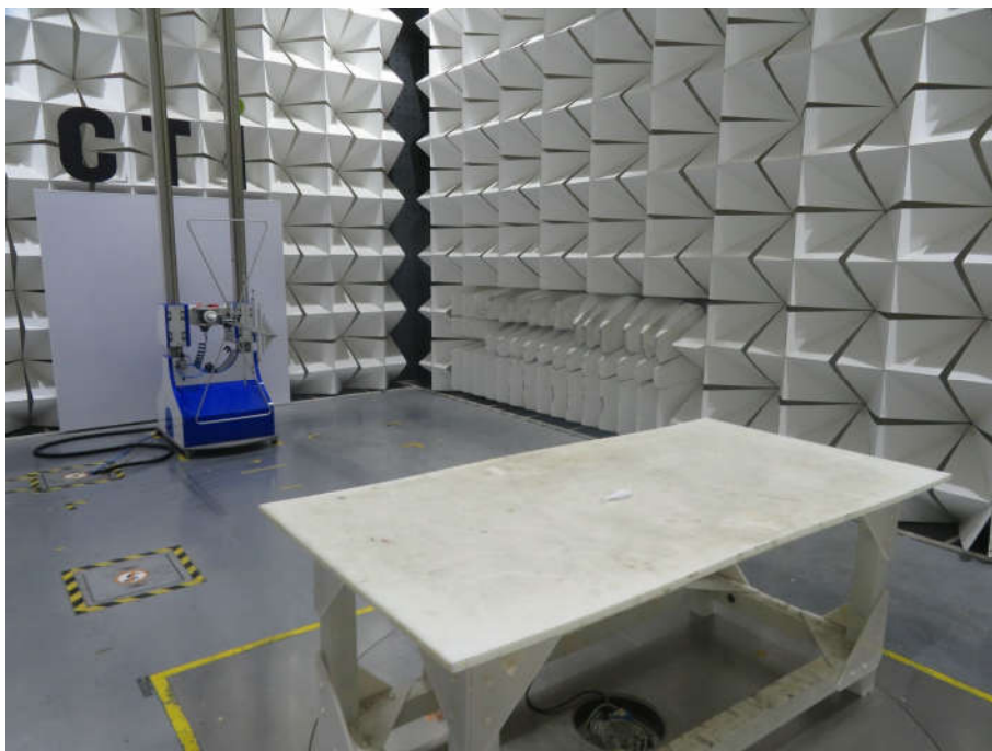
Radiated spurious emission Test Setup-2 (30MHz- 1GHz)
