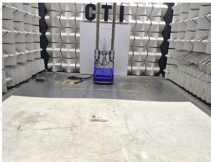
Radiated spurious emission Test Setup-2(Below 1GHz)
