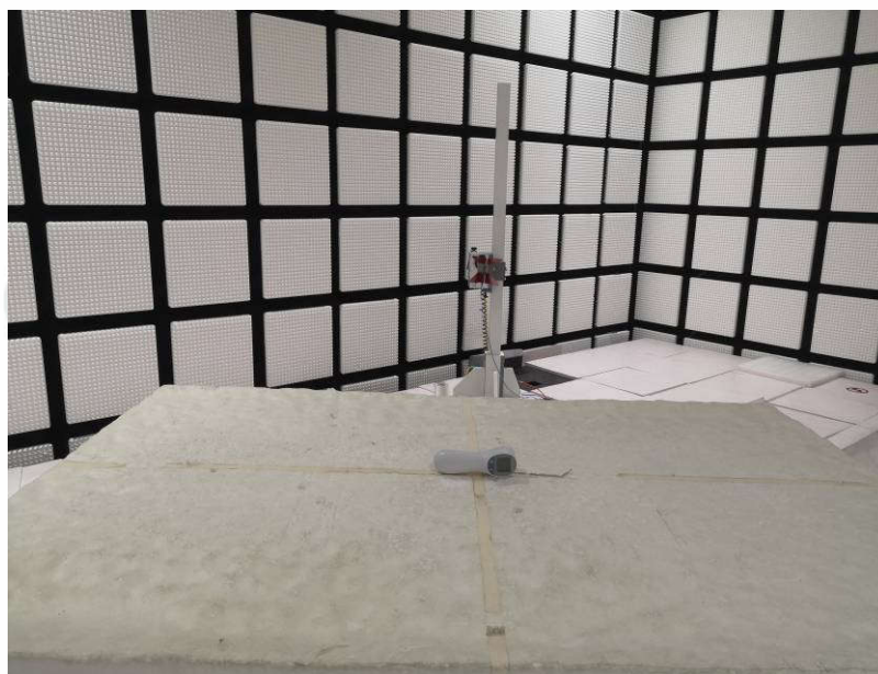
Radiated spurious emission Test Setup-3(Above 1GHz)
