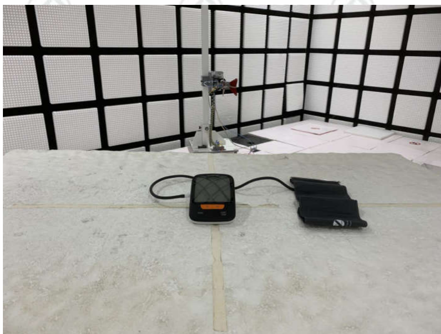
Radiated spurious emission Test Setup-2(Above 1GHz)
