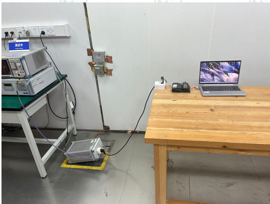
Conducted Emissions Test Setup
