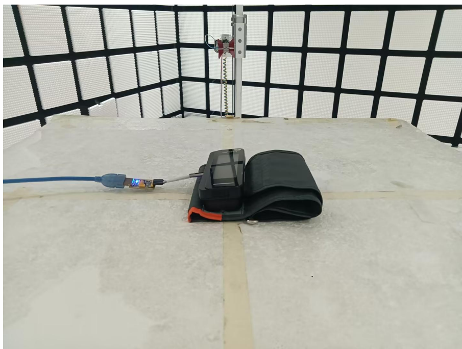
Radiated spurious emission Test Setup-2(Above 1GHz)
