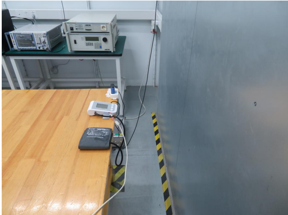
Description: Side View of AC Conducted Emission Test Setup
