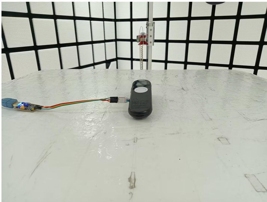
Radiated spurious emission Test Setup-4(Above 1GHz)
