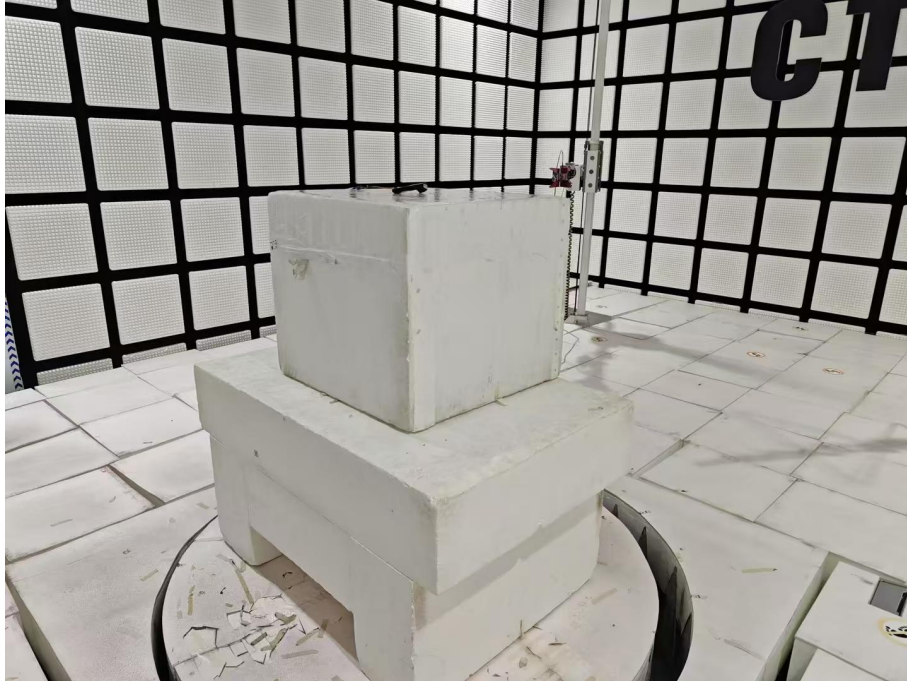
Radiated spurious emission Test Setup-3(Above 1GHz)
