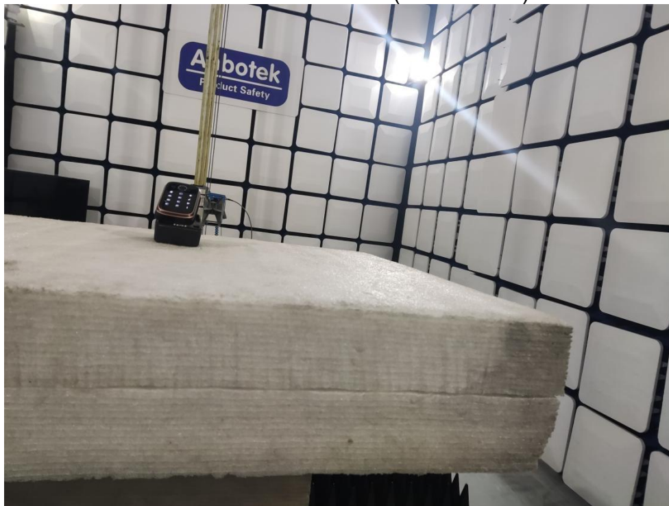
Radiation Emission Test (above 1GHz)
