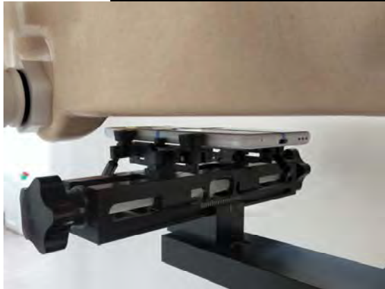
Fig.7 EUT Front side to flat phantom
