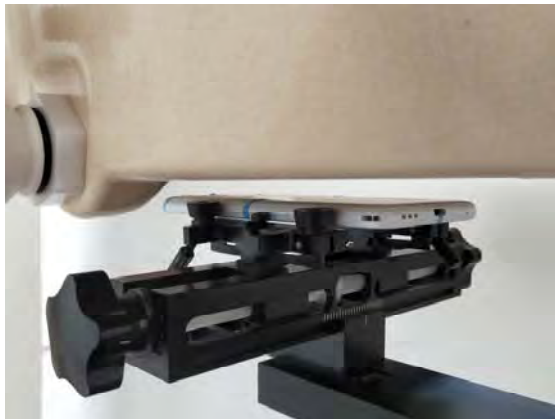
Fig.8 EUT Back side to flat phantom
