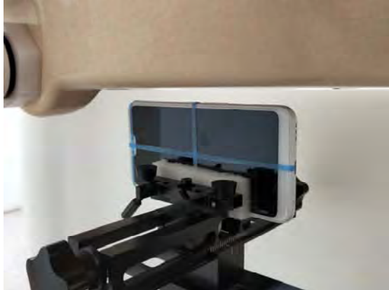
Fig.12 EUT Right side to flat phantom
