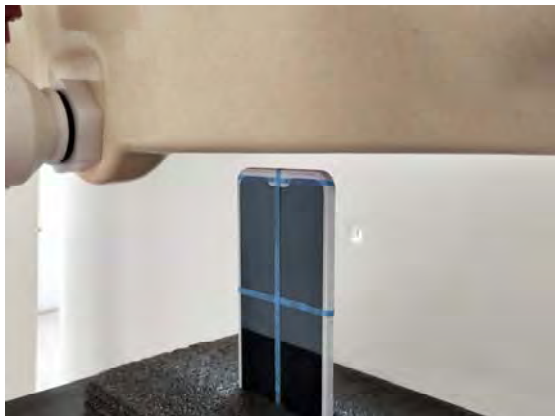
Fig.14 EUT Top side to flat phantom
