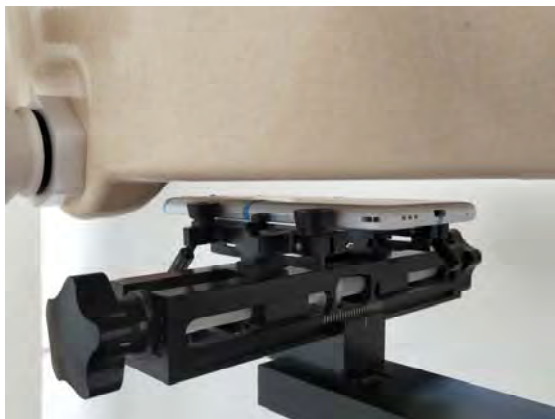
Fig.10 EUT Back side to flat phantom
