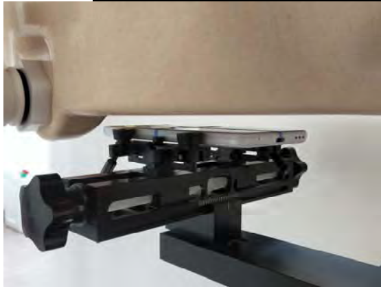
Fig.9 EUT Front side to flat phantom
