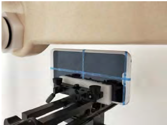
Fig.13 EUT Left side to flat phantom
