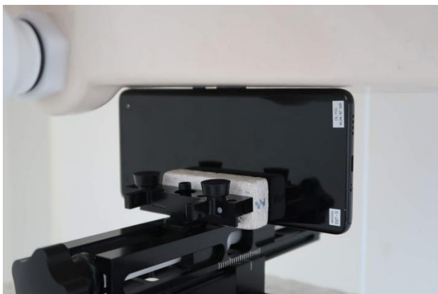
Right Side, Test Separation 0 mm
