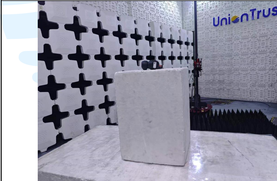
Radiated emission Test Setup (Above 1 GHz)
