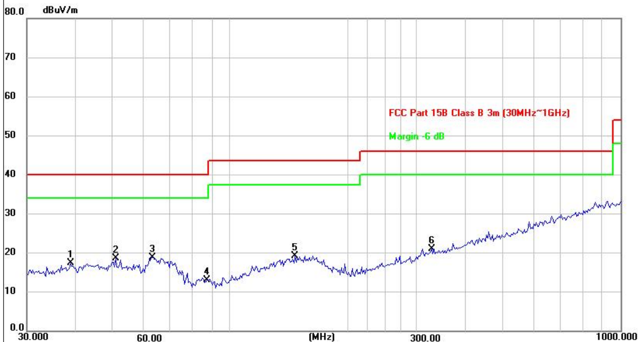
Antennal Polarity& Test Distance: Vertical at 3m
