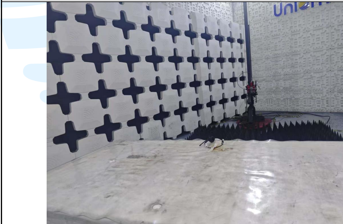
Radiated emission Test Setup-2 (Above 1 GHz)
