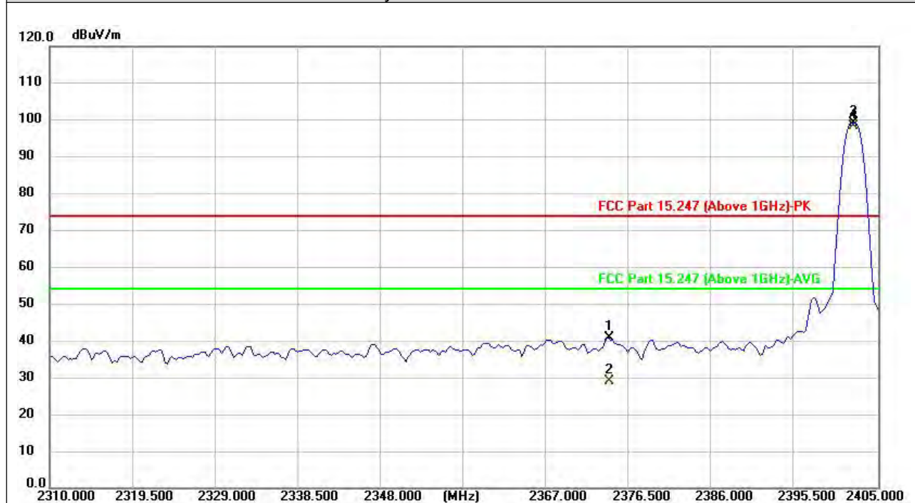
Antenna Polarity& Test distance: Horizontal at 3 M
