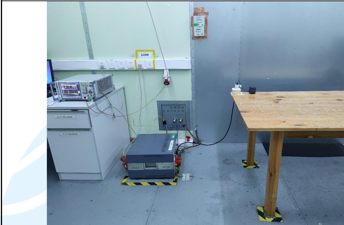
AC Power Line Conducted Emission Test Setup
