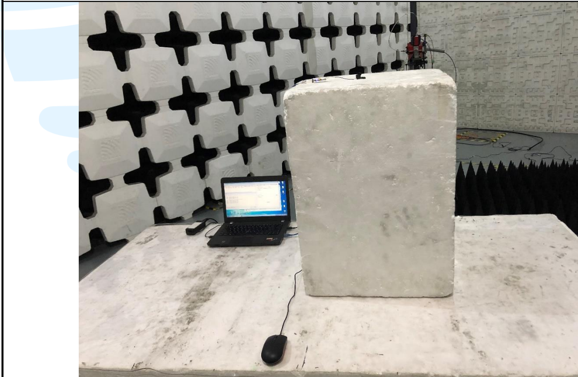
Radiated emission Test Setup (Above 1 GHz) _Left earbuds
