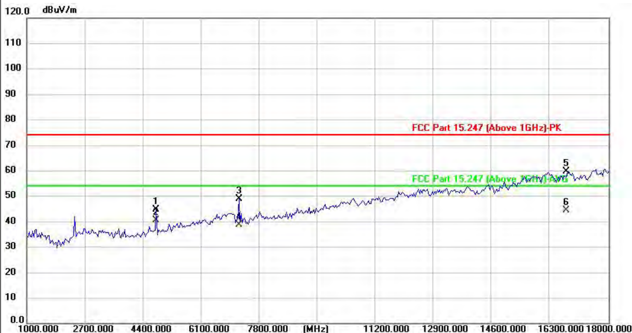
Antennal Polarity& Test distance: Horizontal at 3 M
