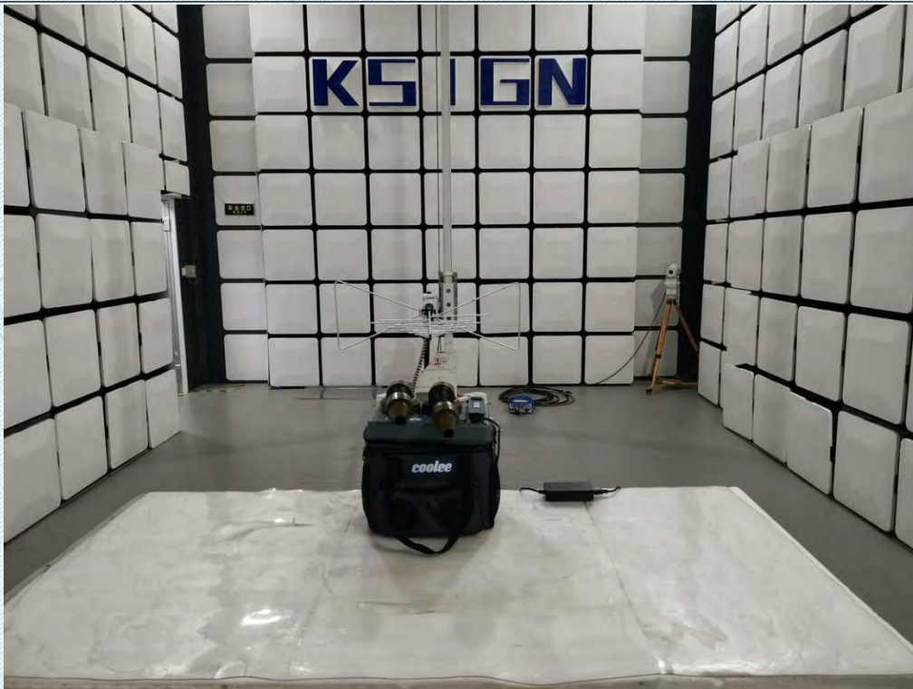
Emissions in restricted frequency bands (below 1GHz)
