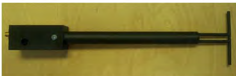
Figure 1 – MVG COMOSAR Validation Dipole
