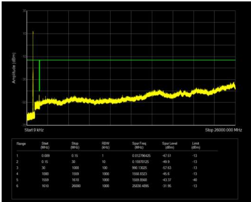
Band13 QPSK BW=5MHz Channel=23255 RB Size=25 Position=#0
