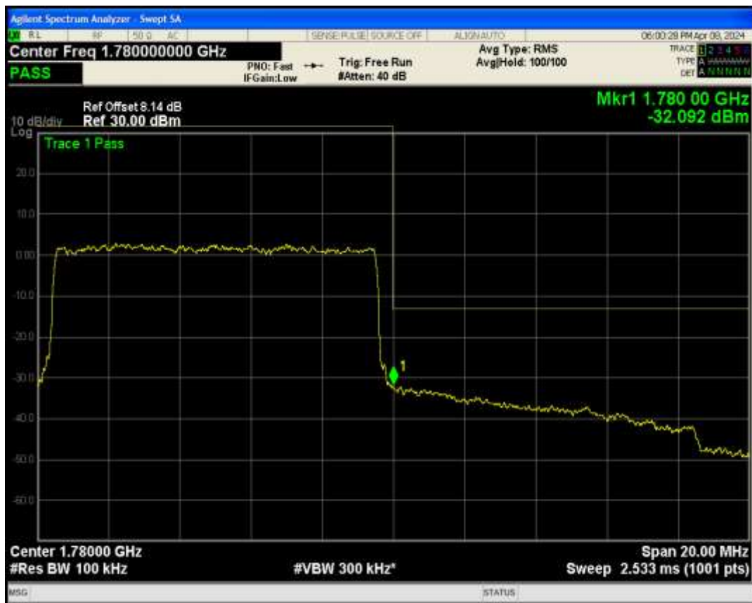
Band66 QPSK BW=15MHz Channel=132047 RB Size=75 Position=#0
