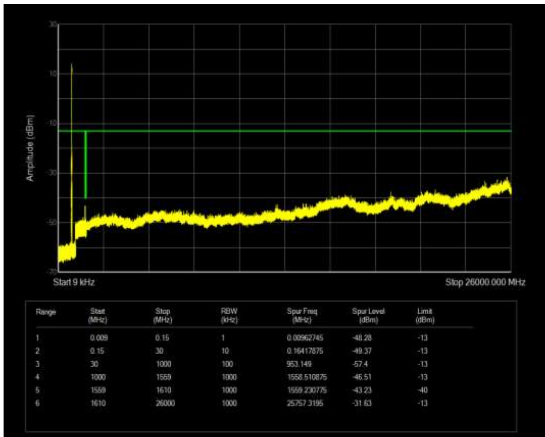
Band13 QAM16 BW=5MHz Channel=23205 RB Size=25 Position=#0
