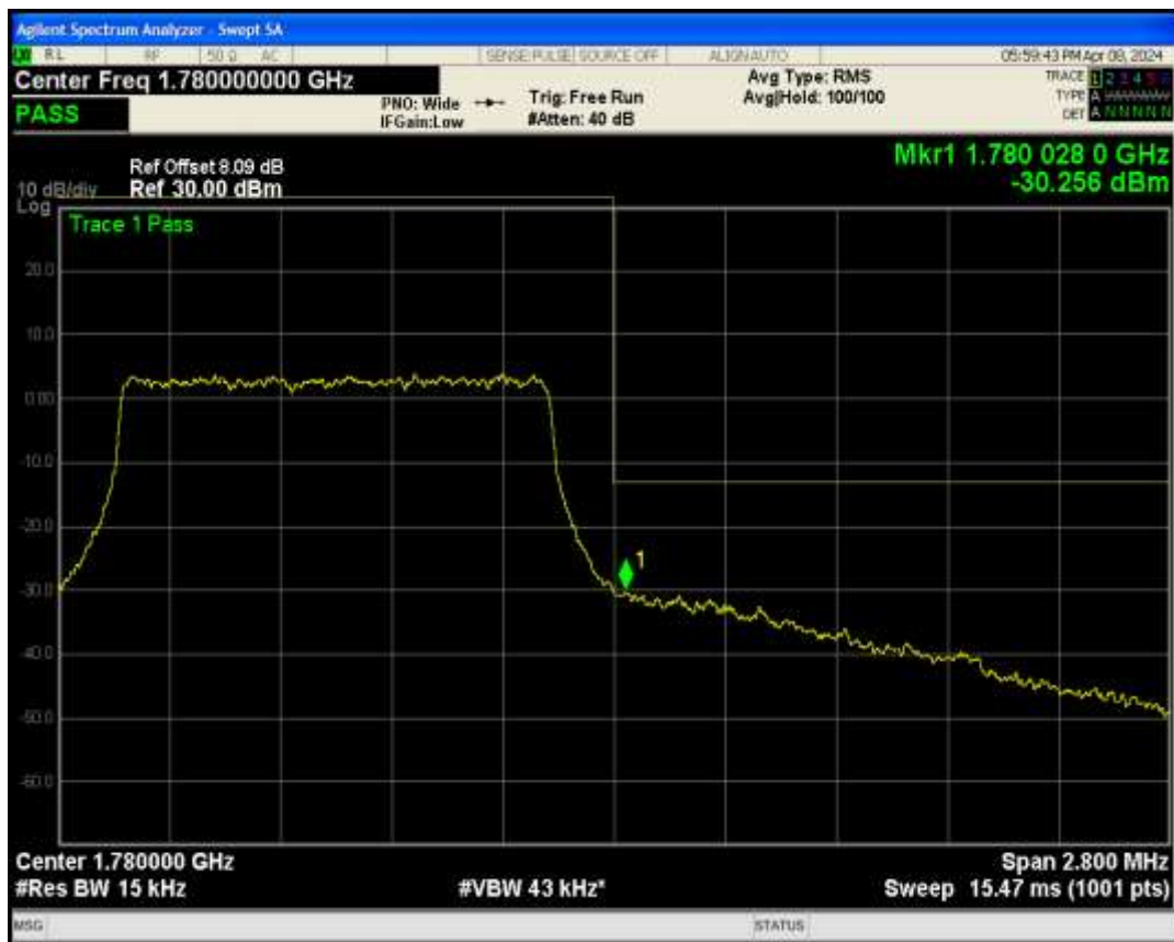
Band66 QPSK BW=3MHz Channel=131987 RB Size=15 Position=#0
