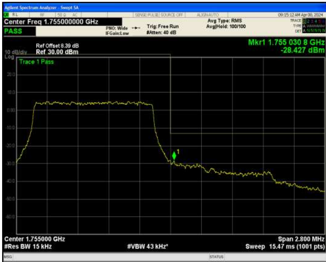
Band4 QAM16 BW=1.4MHz Channel=20393 RB Size=6 Position=#0
