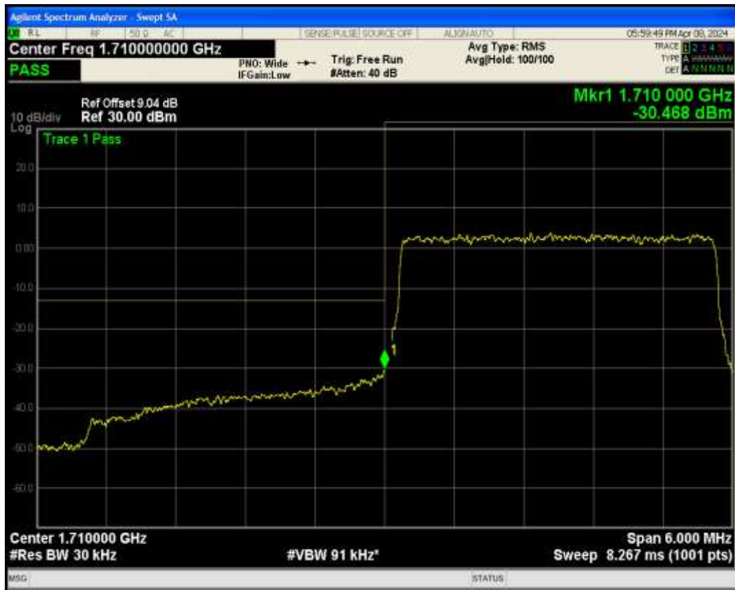
Band66 QAM16 BW=3MHz Channel=131987 RB Size=15 Position=#0
