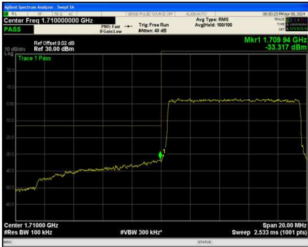
Band66 QPSK BW=10MHz Channel=132622 RB Size=50 Position=#0
