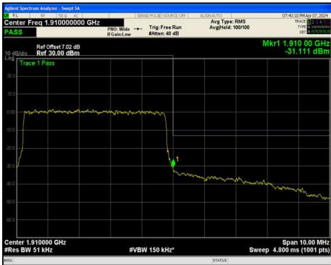
Band2 QPSK BW=10MHz Channel=18650 RB Size=50 Position=#0
