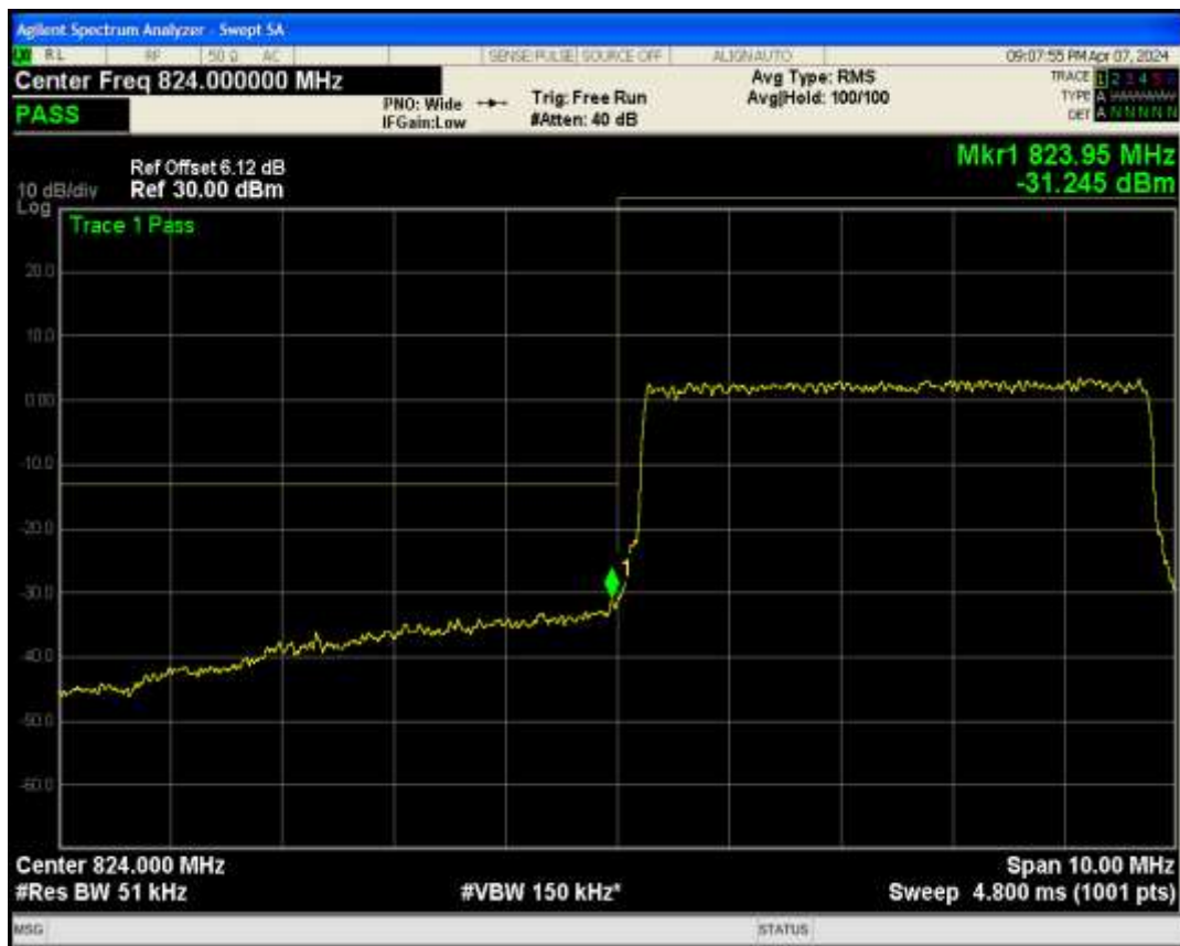
Band5 QPSK BW=5MHz Channel=20625 RB Size=25 Position=#0
