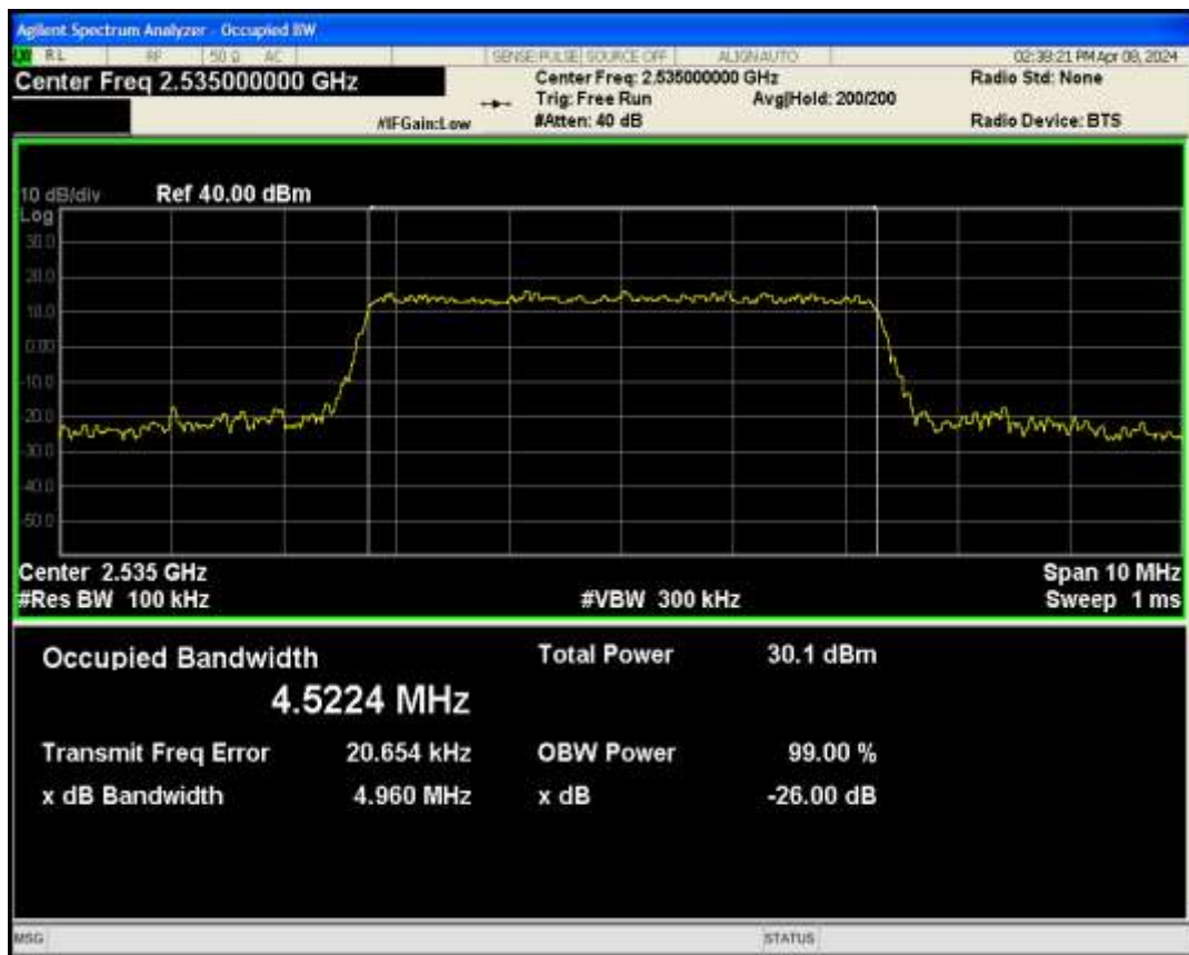
Band7 QPSK BW=15MHz Channel=21100 RB Size=75 Position=#0
