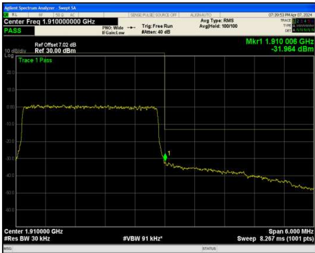
Band2 QPSK BW=5MHz Channel=18625 RB Size=25 Position=#0
