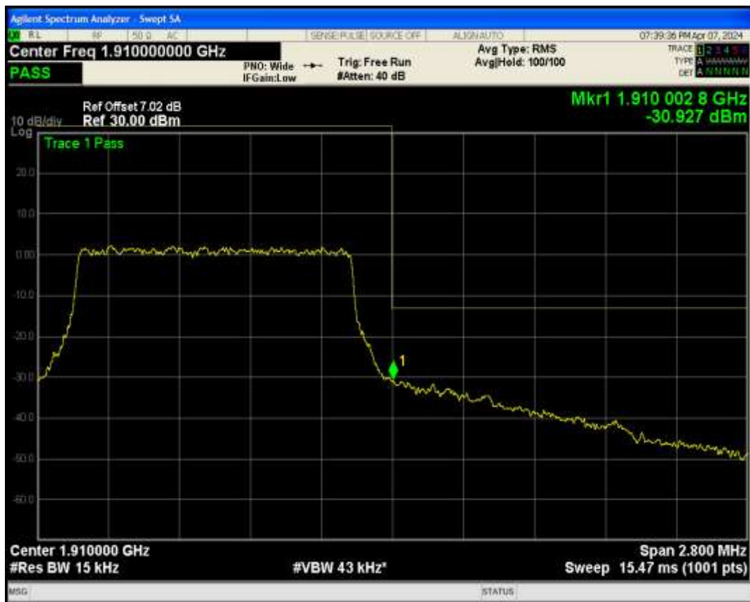
Band2 QPSK BW=3MHz Channel=18615 RB Size=15 Position=#0
