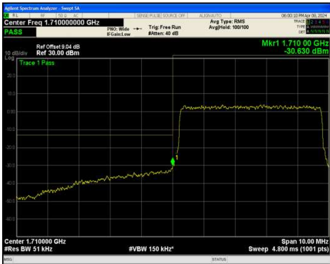
Band66 QPSK BW=5MHz Channel=132647 RB Size=25 Position=#0
