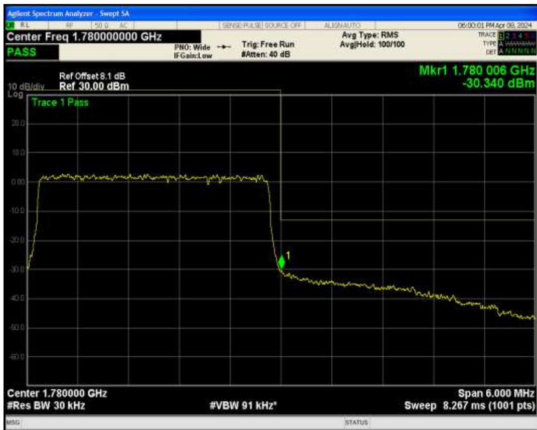
Band66 QPSK BW=5MHz Channel=131997 RB Size=25 Position=#0
