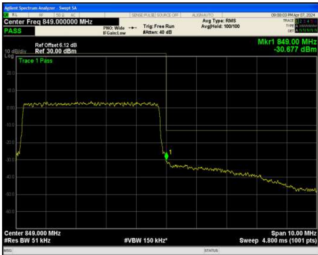
Band5 QPSK BW=10MHz Channel=20450 RB Size=50 Position=#0
