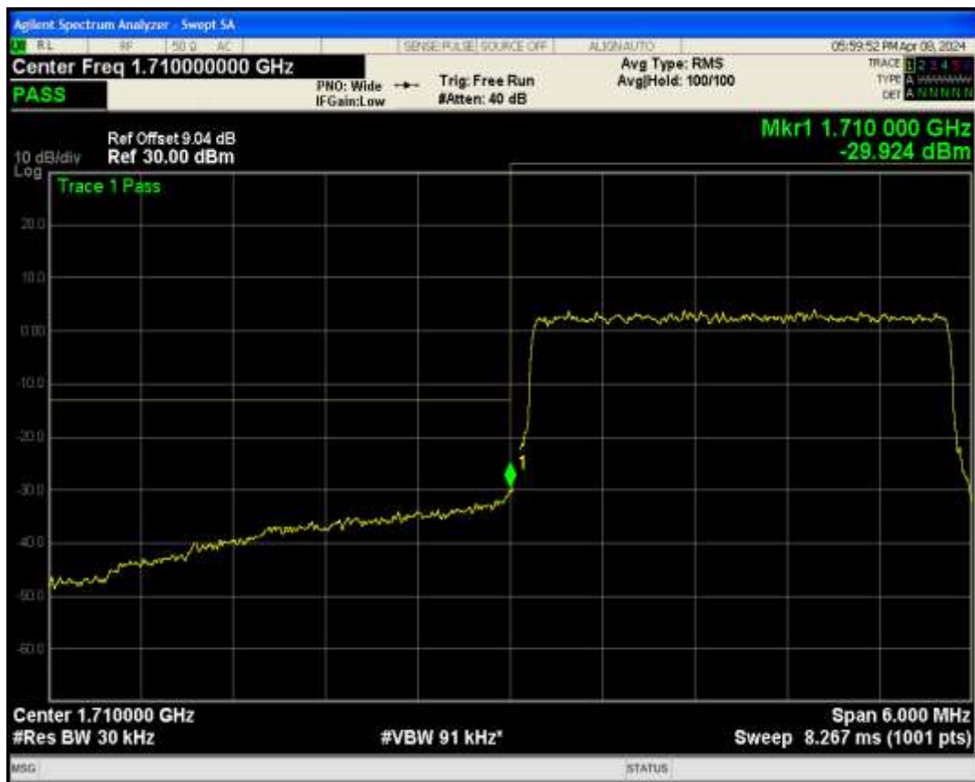
Band66 QPSK BW=3MHz Channel=132657 RB Size=15 Position=#0
