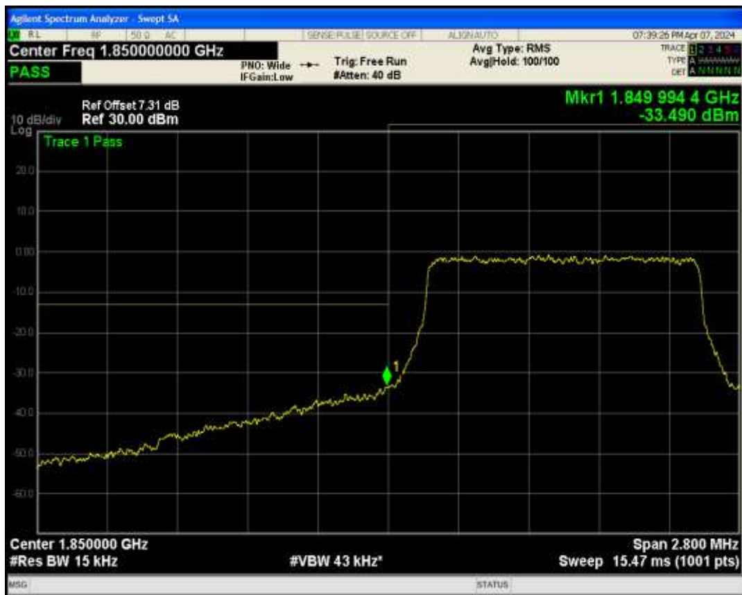
Band2 QPSK BW=1.4MHz Channel=19193 RB Size=6 Position=#0
