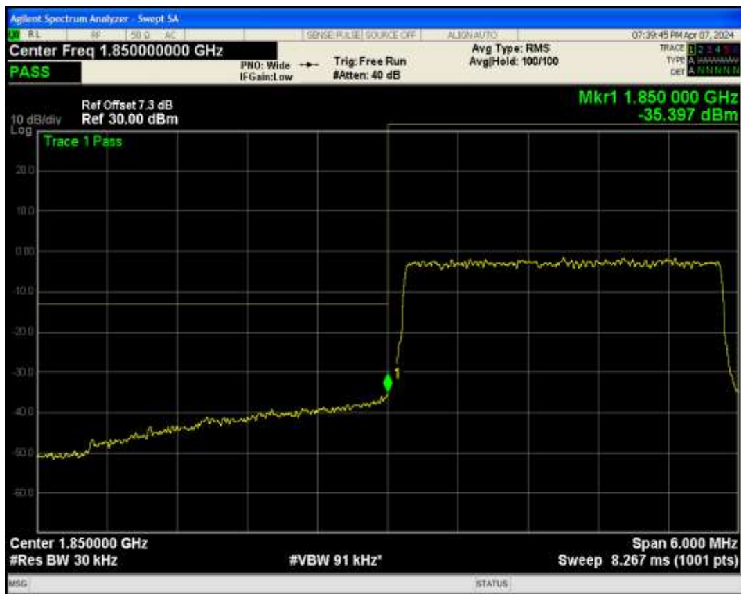
Band2 QPSK BW=3MHz Channel=19185 RB Size=15 Position=#0
