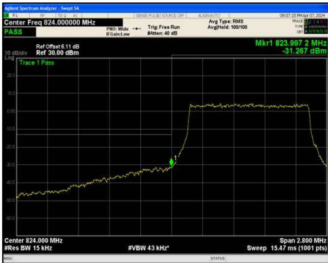
Band5 QPSK BW=1.4MHz Channel=20643 RB Size=6 Position=#0
