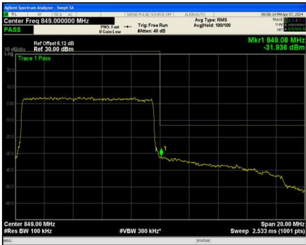
Band66 QPSK BW=1.4MHz Channel=131979 RB Size=6 Position=#0
