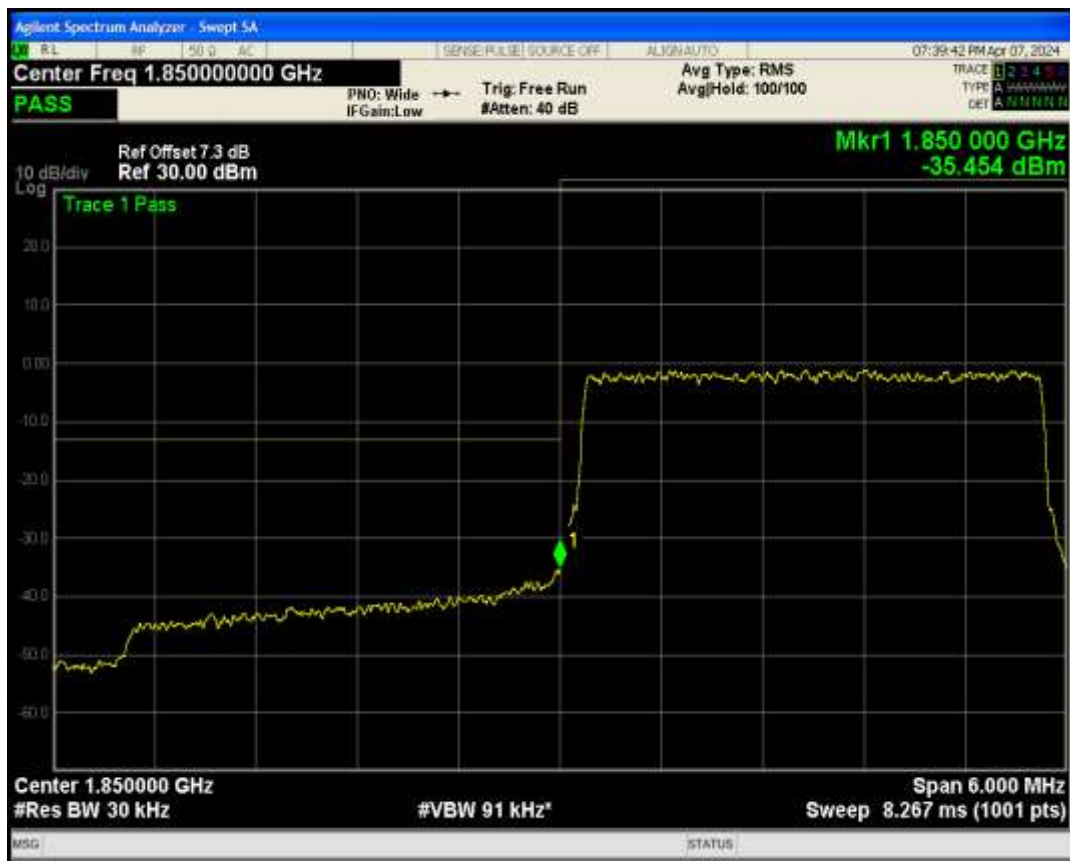
Band2 QAM16 BW=3MHz Channel=18615 RB Size=15 Position=#0
