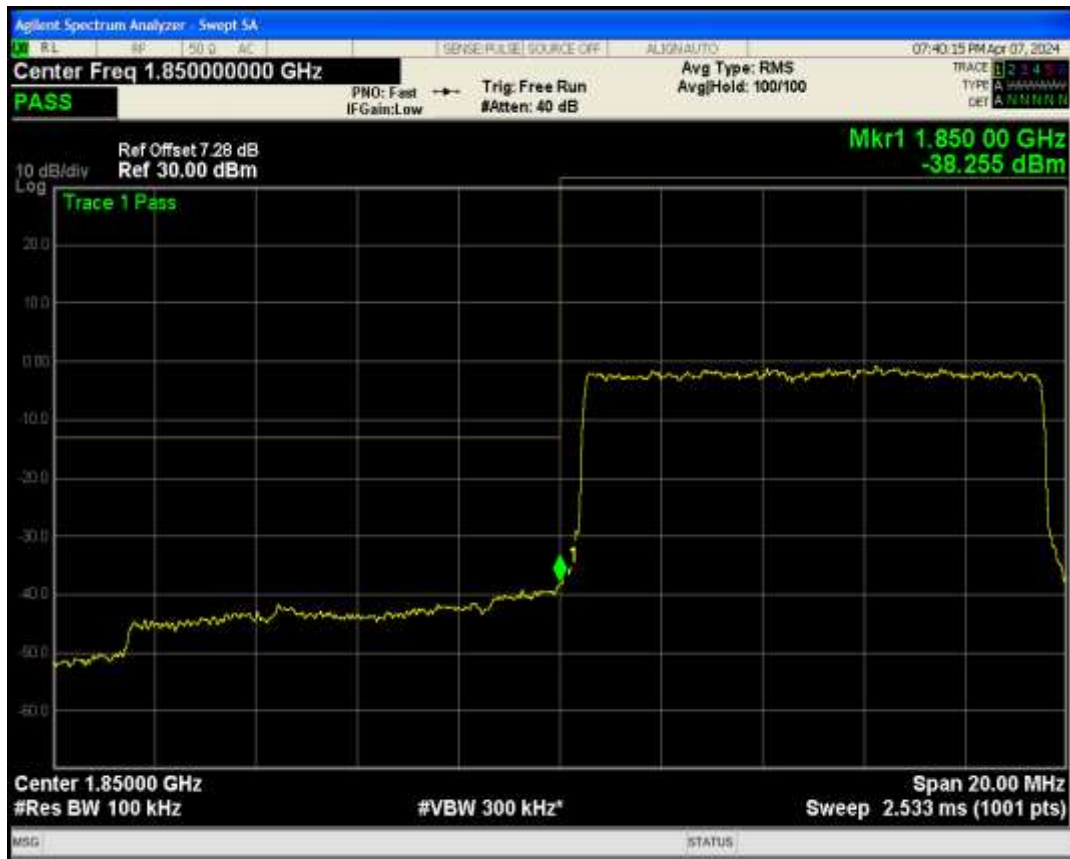
Band2 QPSK BW=10MHz Channel=19150 RB Size=50 Position=#0
