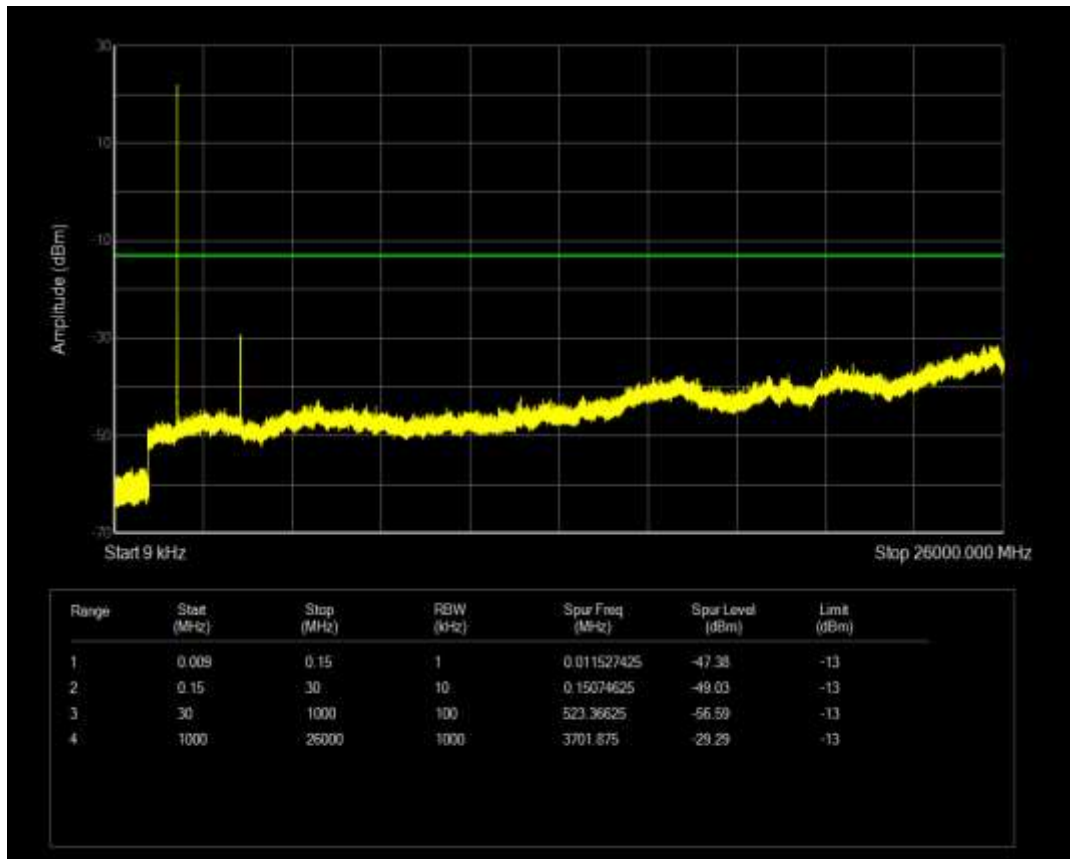
Band2 QAM16 BW=1.4MHz Channel=18607 RB Size=6 Position=#0
