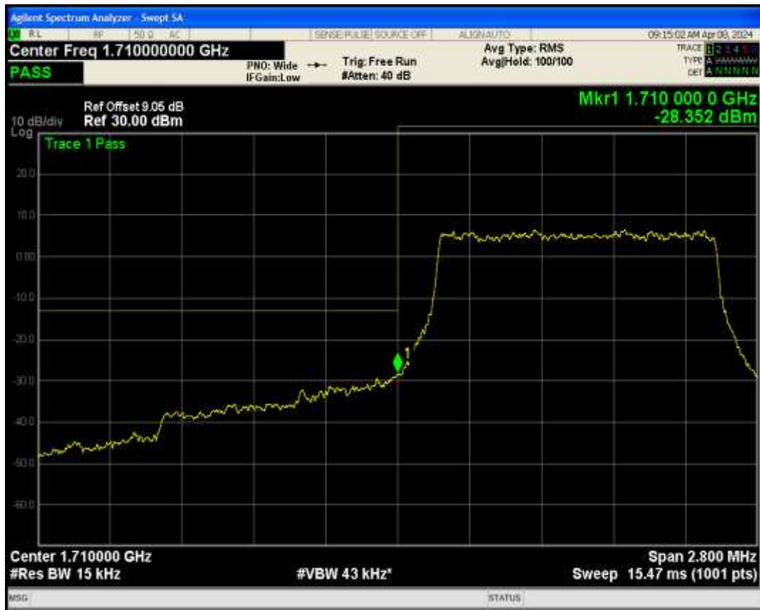
Band4 QAM16 BW=1.4MHz Channel=19957 RB Size=6 Position=#0
