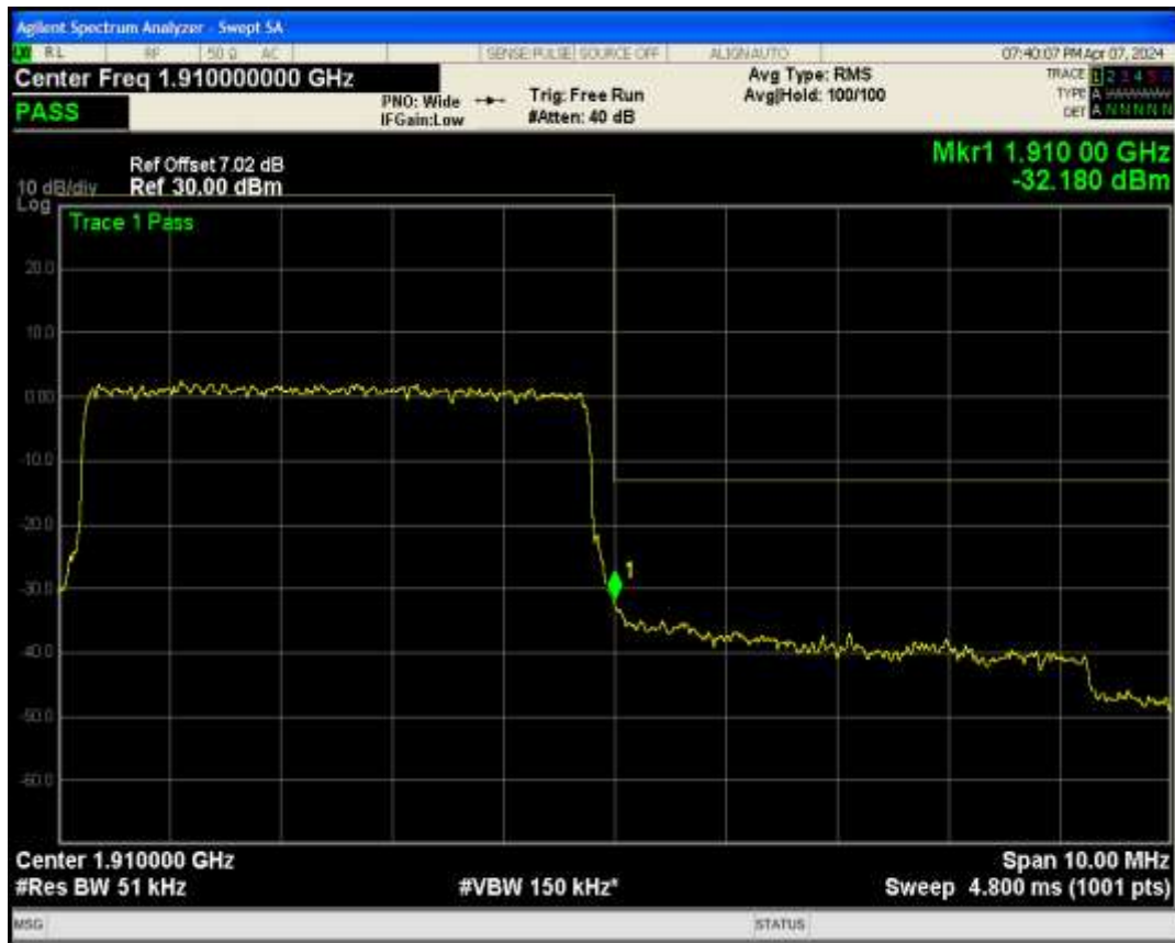
Band2 QAM16 BW=5MHz Channel=19175 RB Size=25 Position=#0
