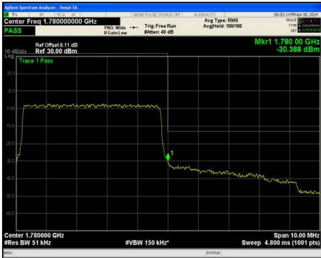
Band66 QAM16 BW=5MHz Channel=132647 RB Size=25 Position=#0
