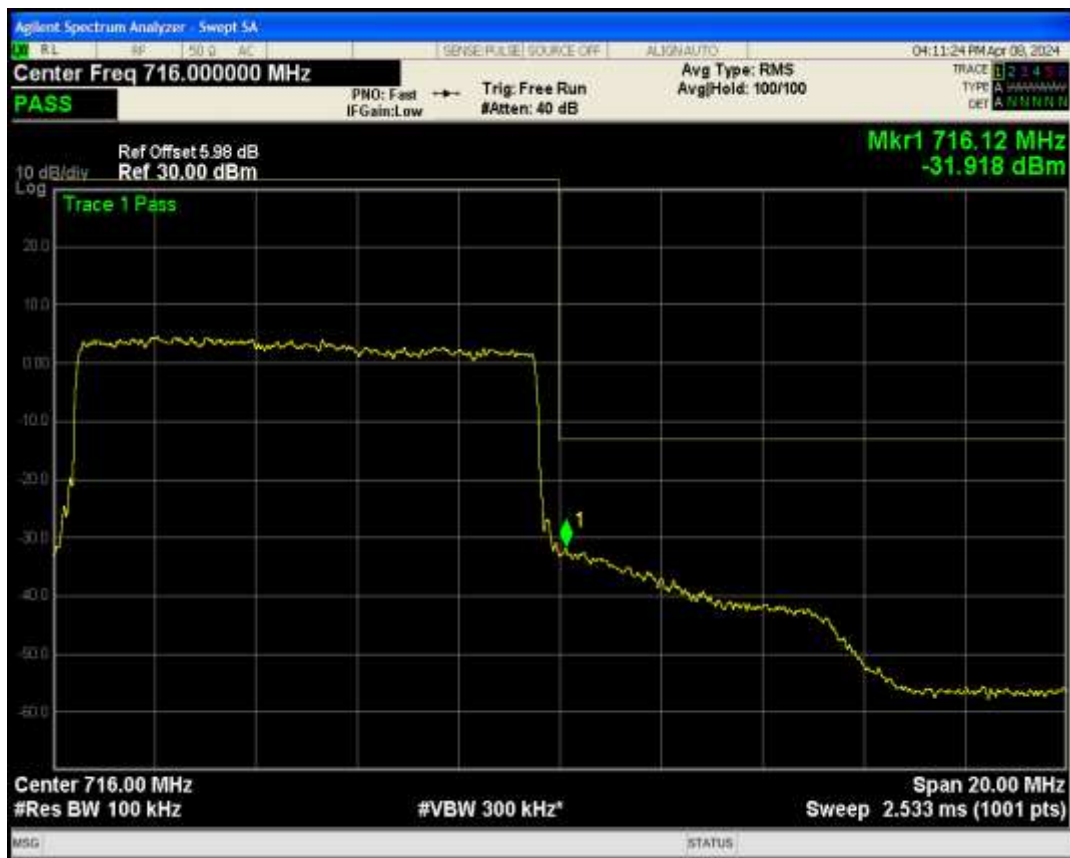
Band2 QPSK BW=1.4MHz Channel=18607 RB Size=6 Position=#0
