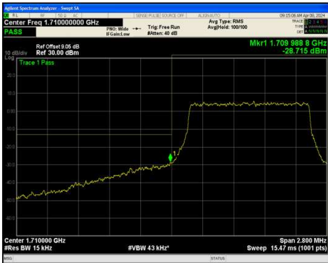
Band4 QPSK BW=1.4MHz Channel=20393 RB Size=6 Position=#0
