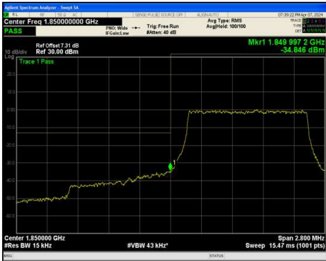
Band2 QAM16 BW=1.4MHz Channel=18607 RB Size=6 Position=#0
