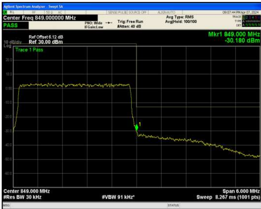
Band5 QPSK BW=5MHz Channel=20425 RB Size=25 Position=#0
