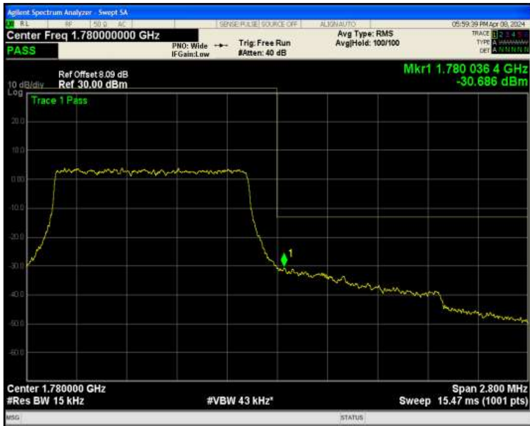
Band66 QAM16 BW=1.4MHz Channel=132665 RB Size=6 Position=#0
