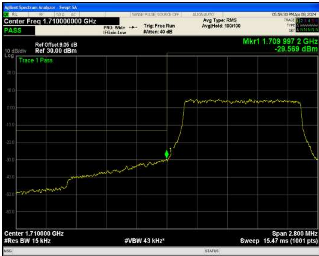
Band66 QAM16 BW=1.4MHz Channel=131979 RB Size=6 Position=#0
