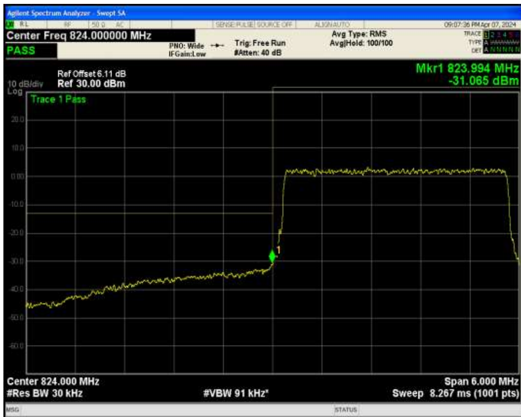
Band5 QPSK BW=3MHz Channel=20635 RB Size=15 Position=#0
