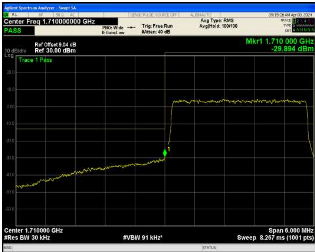
Band4 QPSK BW=3MHz Channel=20385 RB Size=15 Position=#0
