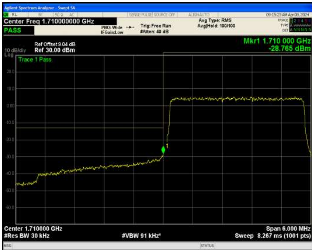
Band4 QAM16 BW=3MHz Channel=19965 RB Size=15 Position=#0
