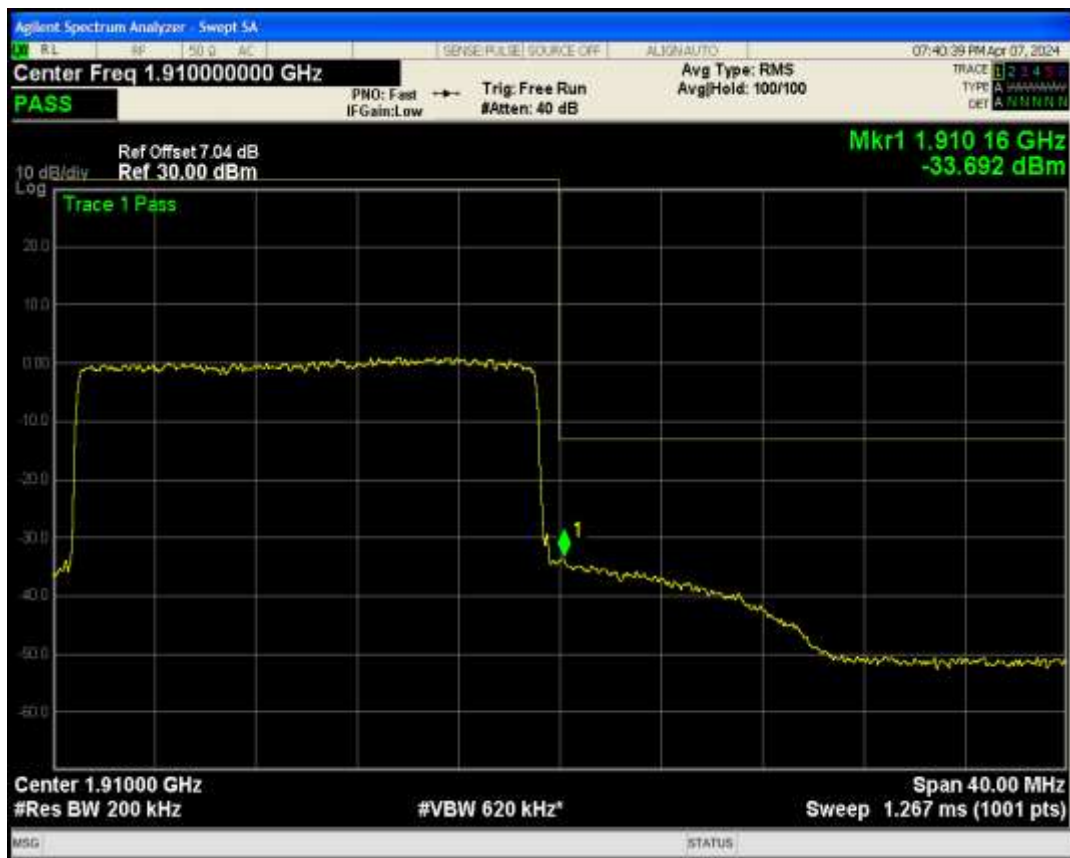
Band38 QPSK BW=5MHz Channel=37775 RB Size=25 Position=#0
