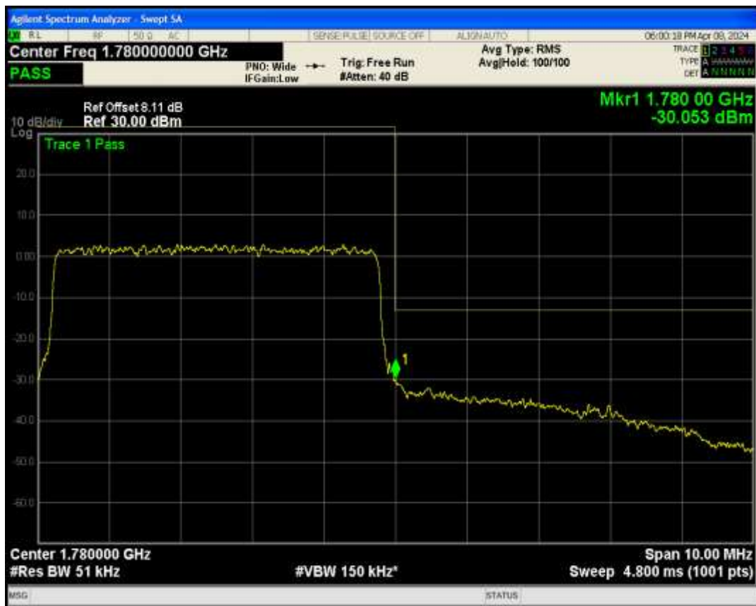
Band66 QPSK BW=10MHz Channel=132022 RB Size=50 Position=#0
