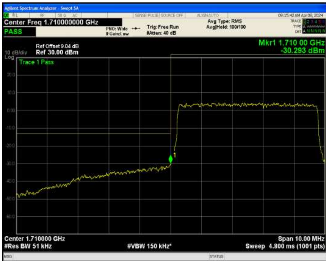
Band4 QPSK BW=5MHz Channel=20375 RB Size=25 Position=#0
