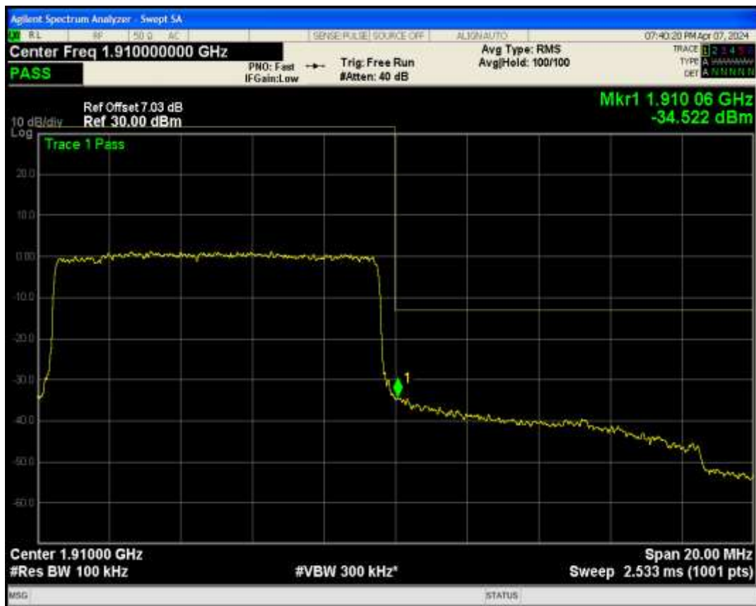
Band2 QPSK BW=15MHz Channel=18675 RB Size=75 Position=#0
