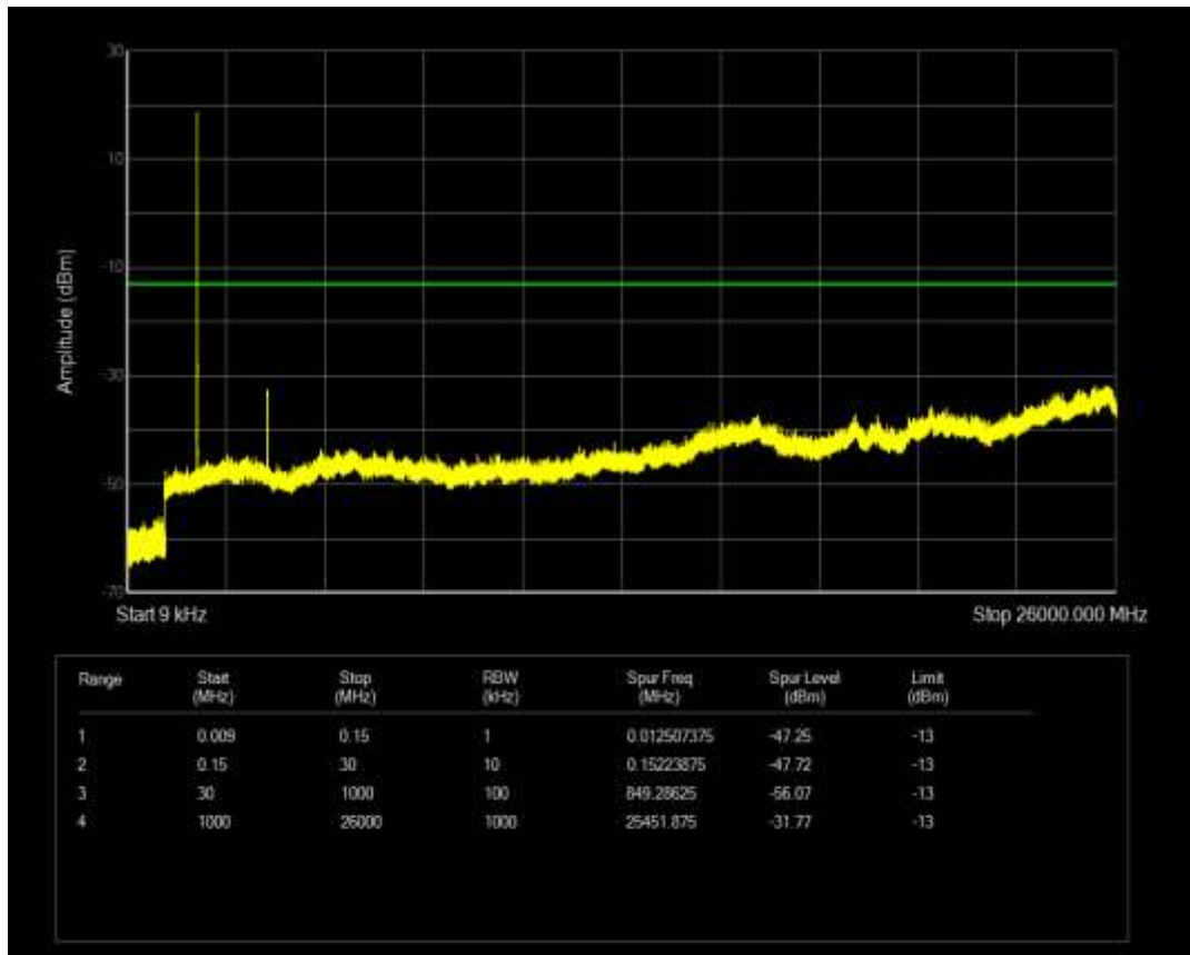
Band2 QAM16 BW=3MHz Channel=18615 RB Size=15 Position=#0
