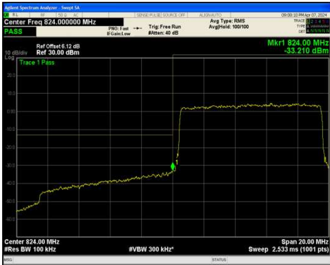
Band5 QPSK BW=10MHz Channel=20600 RB Size=50 Position=#0
