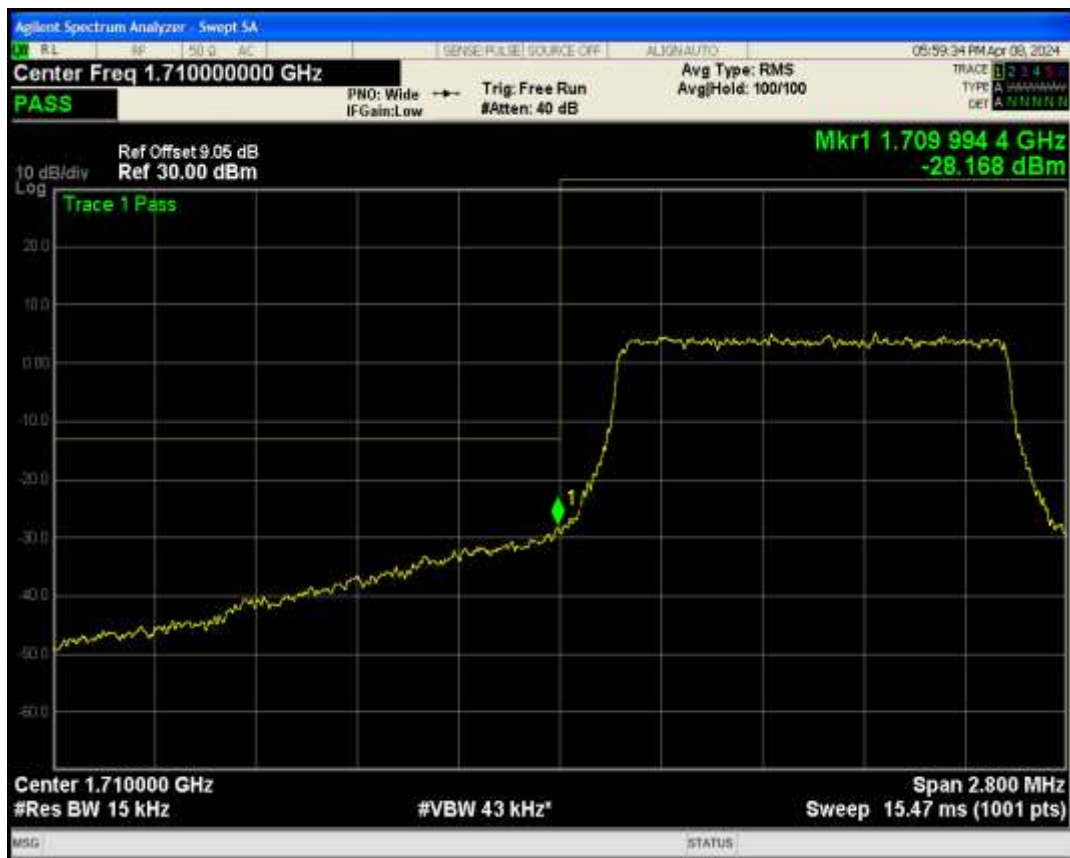
Band66 QPSK BW=1.4MHz Channel=132665 RB Size=6 Position=#0
