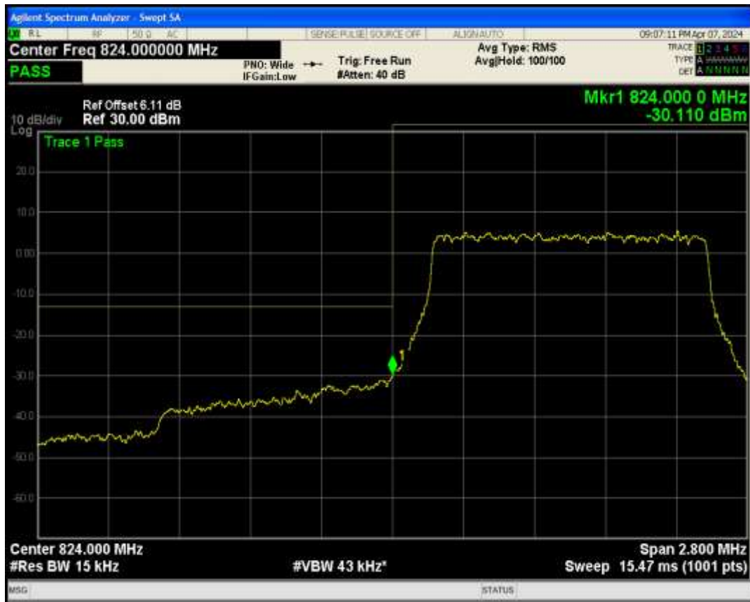
Band5 QAM16 BW=1.4MHz Channel=20407 RB Size=6 Position=#0
