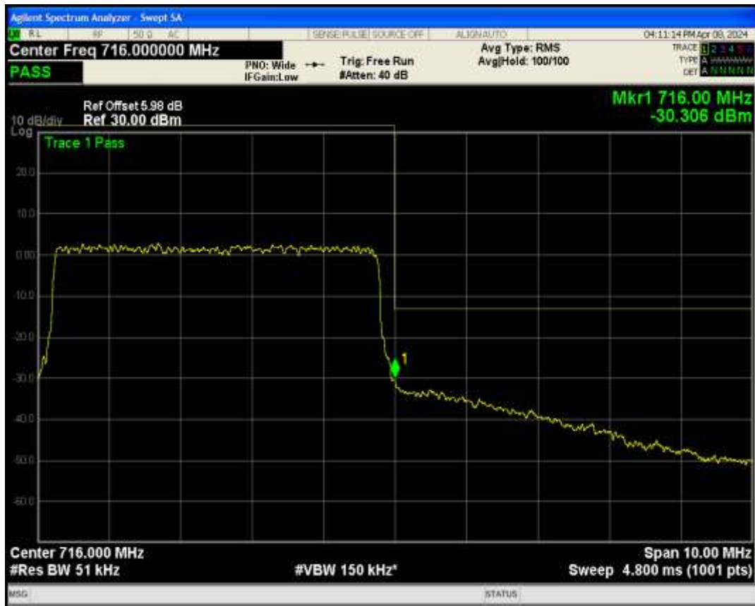
Band17 QPSK BW=10MHz Channel=23800 RB Size=50 Position=#0
