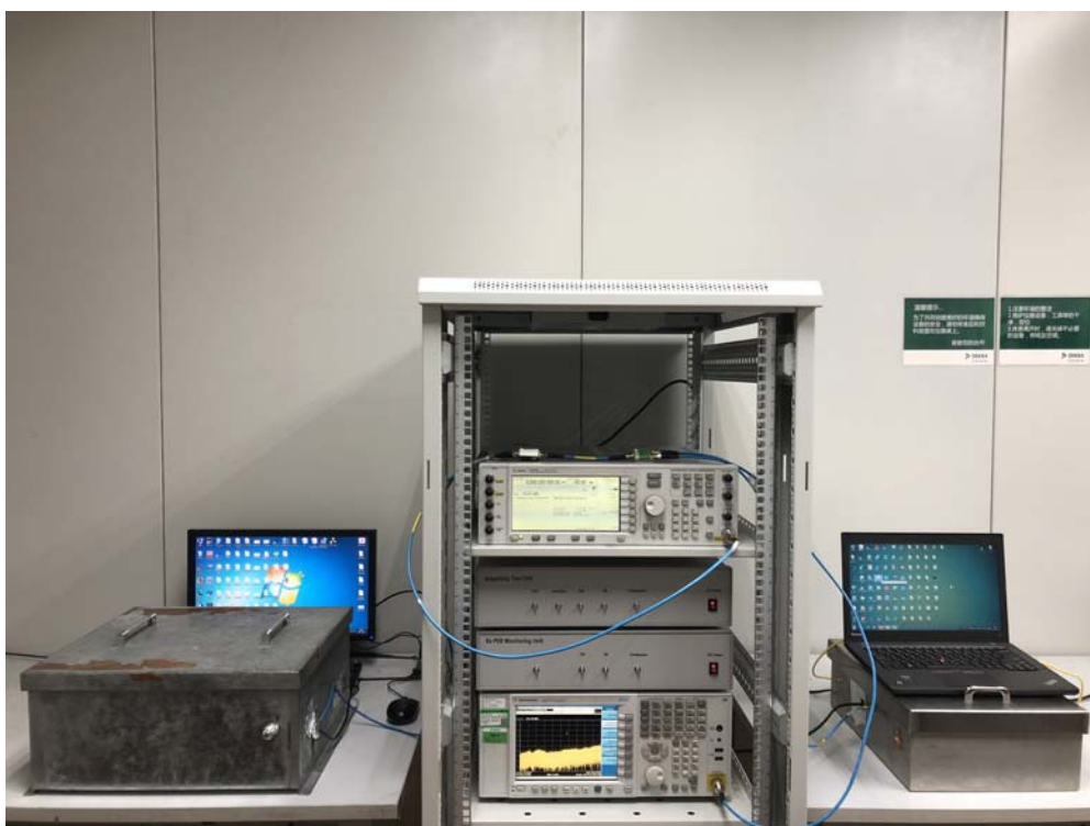
Description: DFS Test Setup
