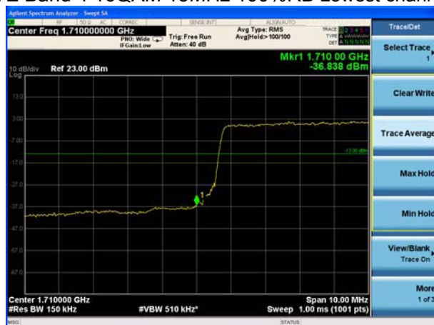
LTE Band 4 16QAM 15MHz 100%RB Lowest channel
