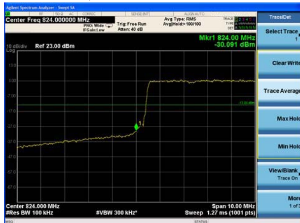
LTE Band 5 16QAM 10MHz 100%RB Lowest channel
