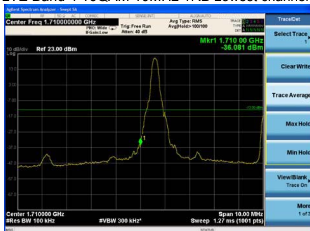
LTE Band 4 16QAM 10MHz 1RB Lowest channel
