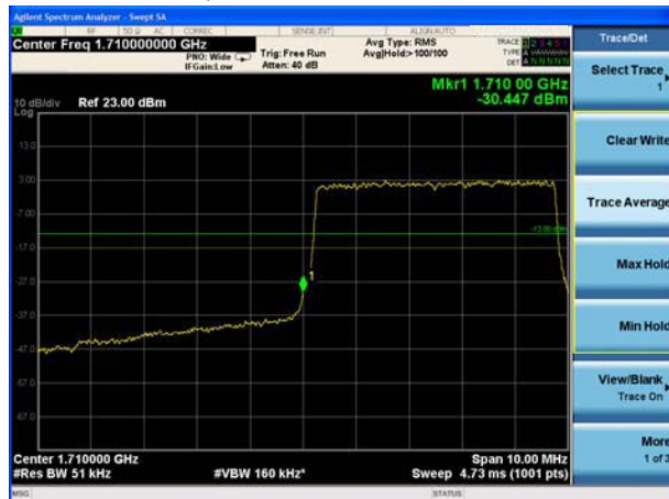
LTE Band 4 16QAM 5MHz 100%RB Lowest channel
