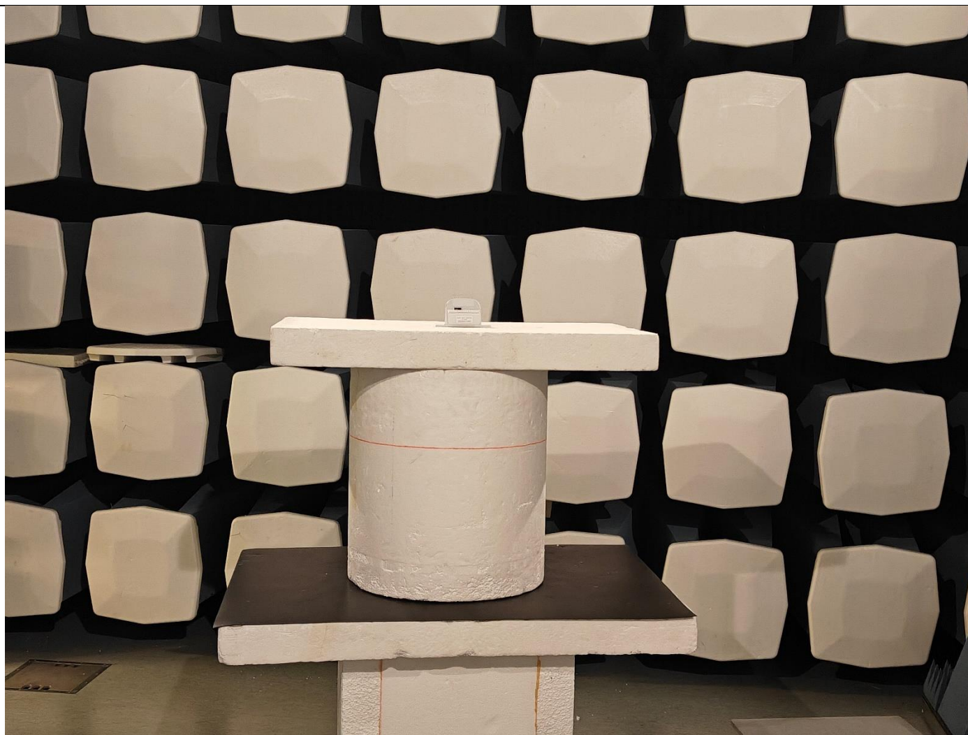
Picture 43, Radiated Spurious Emission, EUT setup, TX, 1 – 26 GHz
