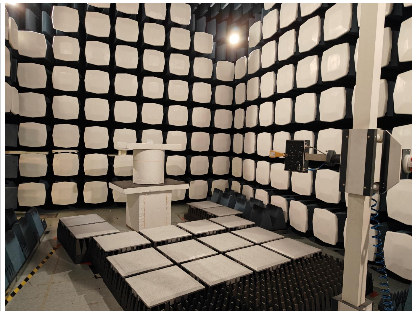
Picture 10, Radiated Spurious Emission, common setup, TX, 18 – 26 GHz, front
