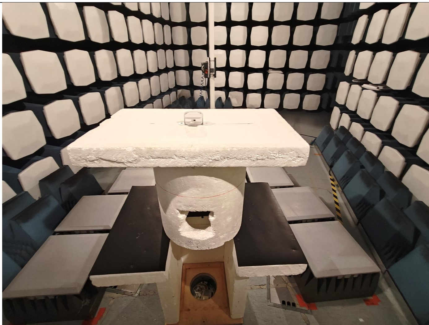
Picture 98, Radiated Spurious Emission, common setup, TX, 18 – 26 GHz, back
