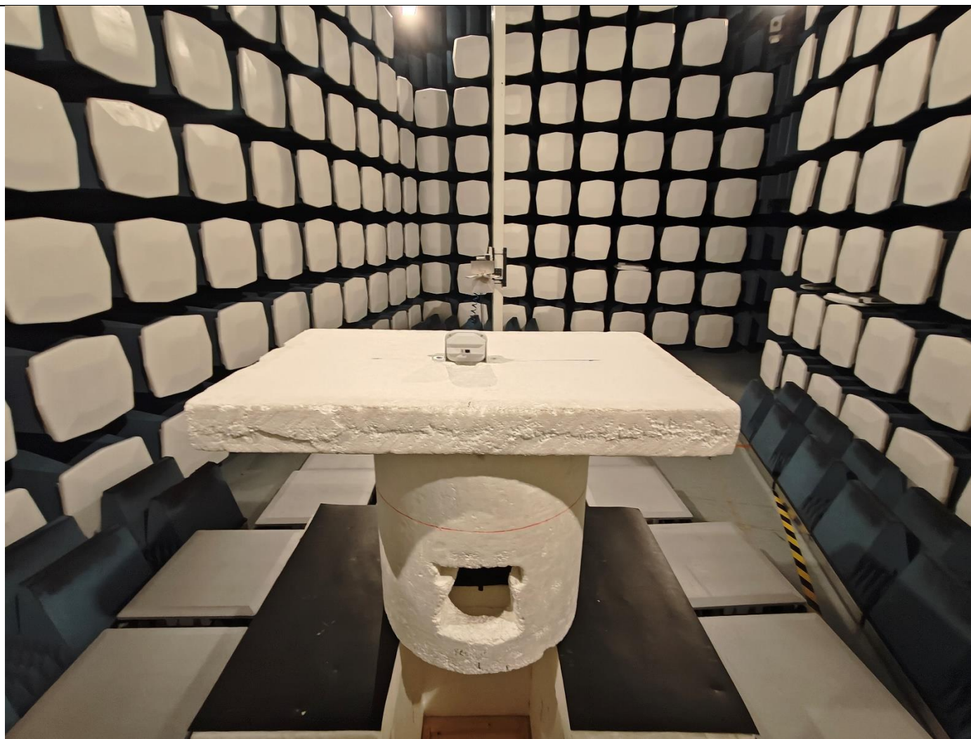
Picture 87, Radiated Spurious Emission, common setup, TX, 1 – 18 GHz, back
