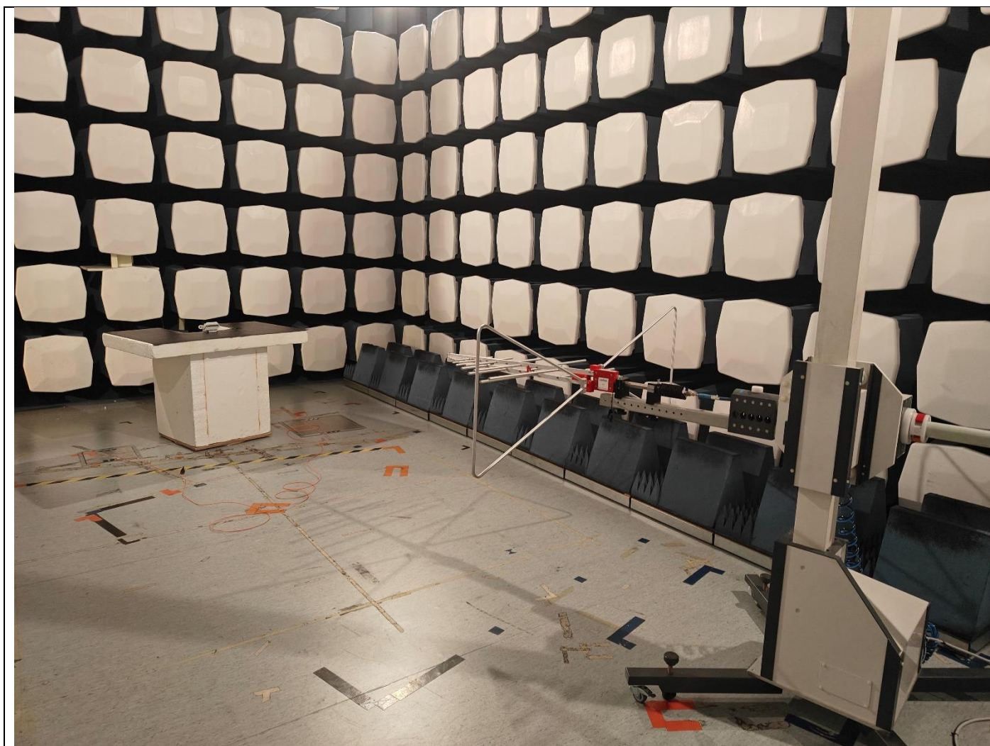
Picture 8, Radiated Spurious Emission, common setup, TX and RX, 30 – 1000 MHz, front
