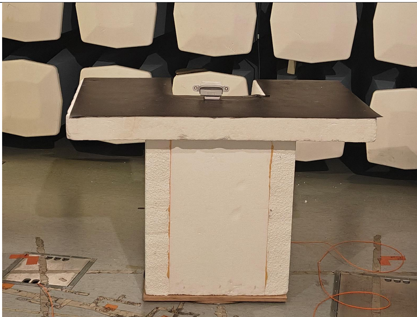
Picture 54, Radiated Spurious Emission, EUT setup, RX, 30 – 1000 MHz
