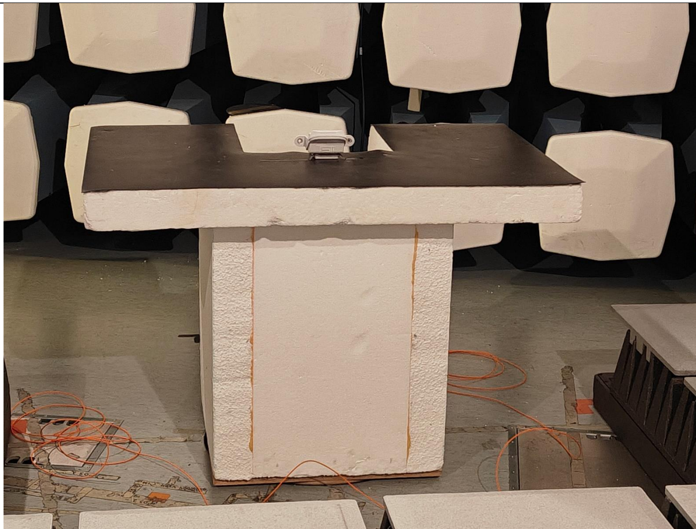
Picture 65, Radiated Spurious Emission, EUT setup, RX, 1 – 40 GHz
