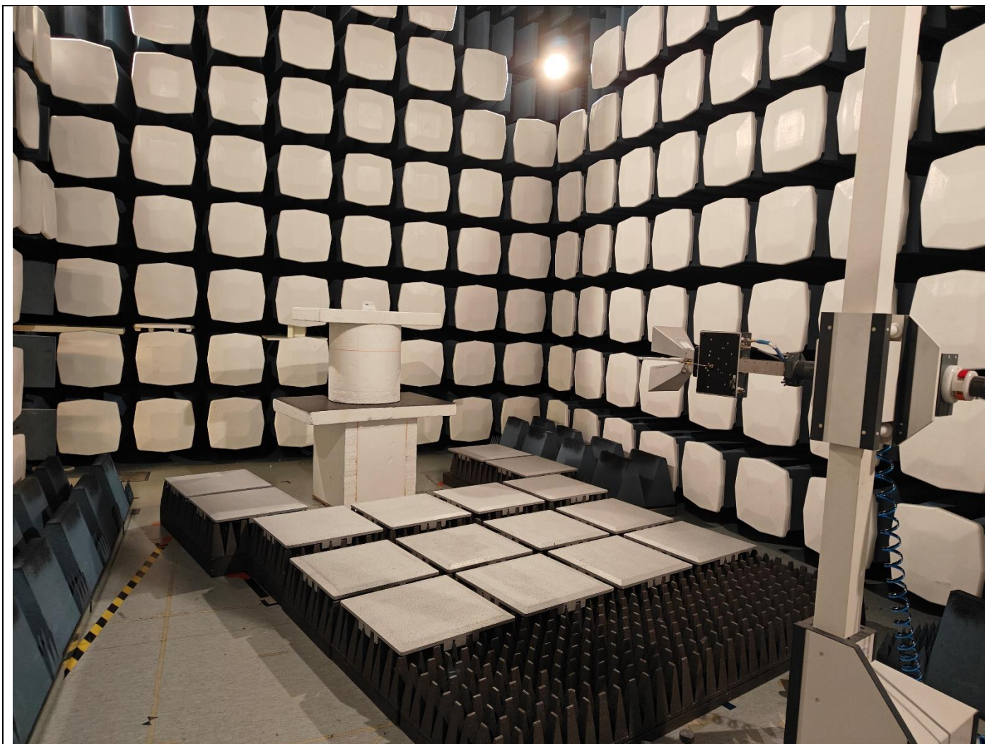
Picture 9, Radiated Spurious Emission, common setup, TX, 1 – 18 GHz, front
