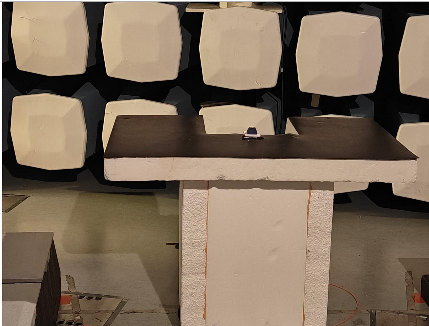
Picture 53, Radiated Spurious Emission, EUT setup, RX, 30 MHz – 12,75 GHz
