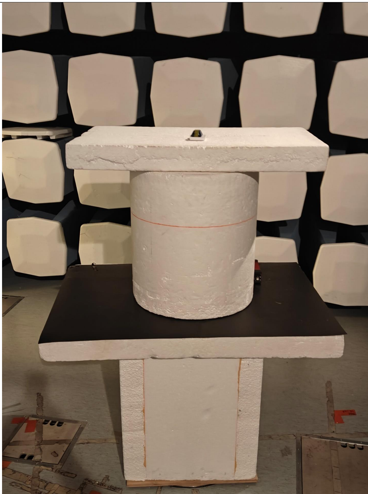
Picture 42, Radiated Spurious Emission, EUT setup, TX, 1 – 26 GHz
