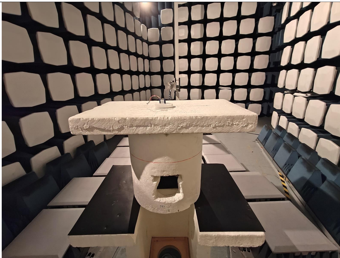
Picture 75, Radiated Spurious Emission, common setup, TX, 1 – 18 GHz, back
