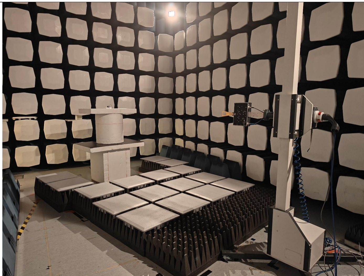
Picture 9, Radiated Spurious Emission, common setup, TX, 18 – 26 GHz, front
