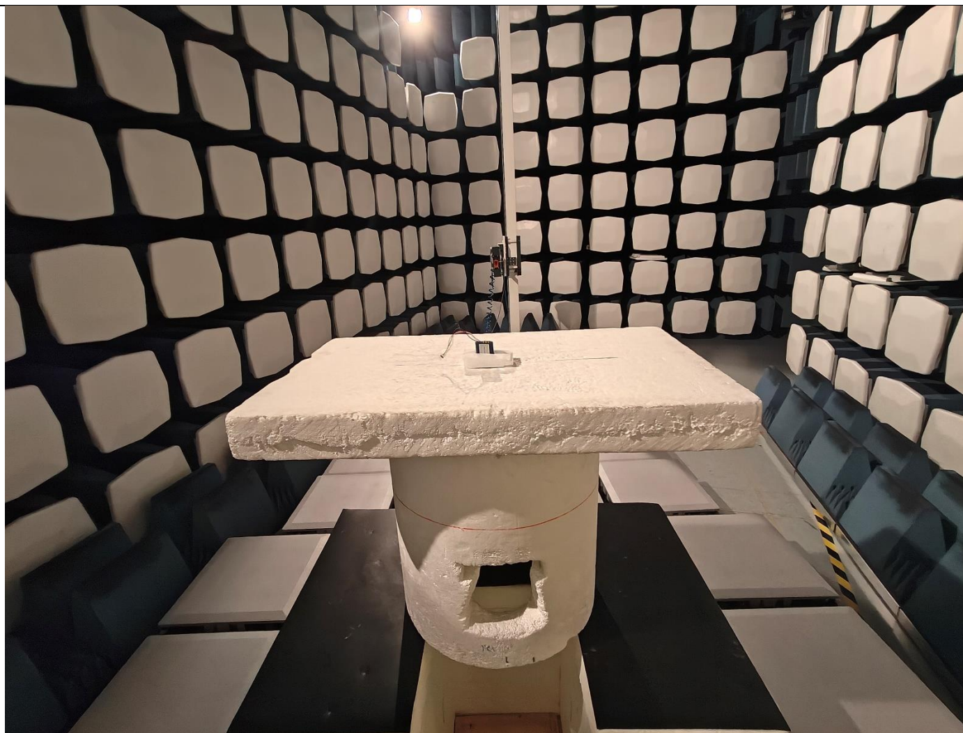
Picture 86, Radiated Spurious Emission, common setup, TX, 18 – 26 GHz, back
