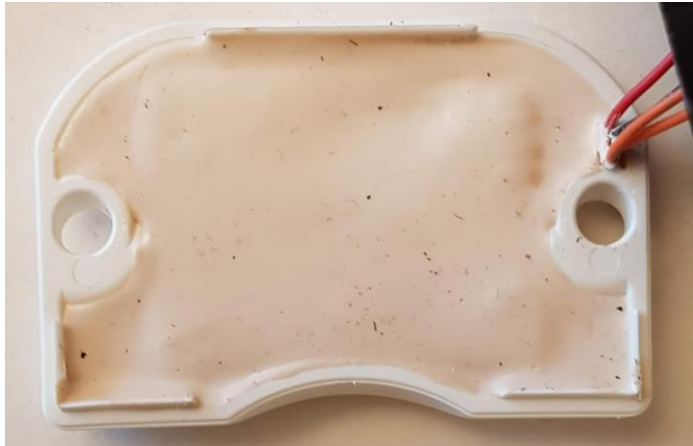
Top lid inside, ISM UHF radio molded into the top lid.
