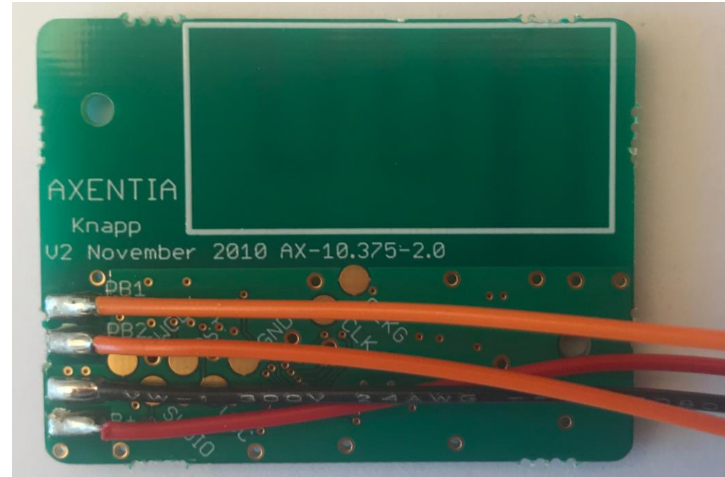
EPM-1000 pcb (molded into the top lid), rear.
