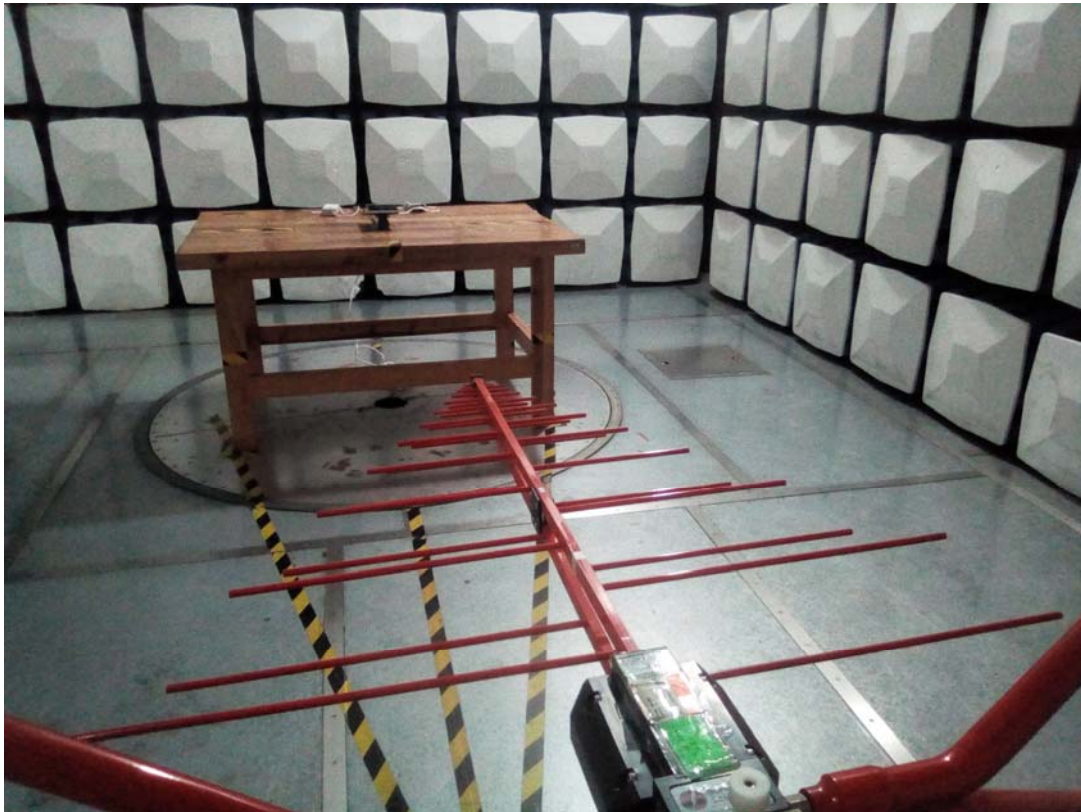
Radiated Emission Below 1GHz View
