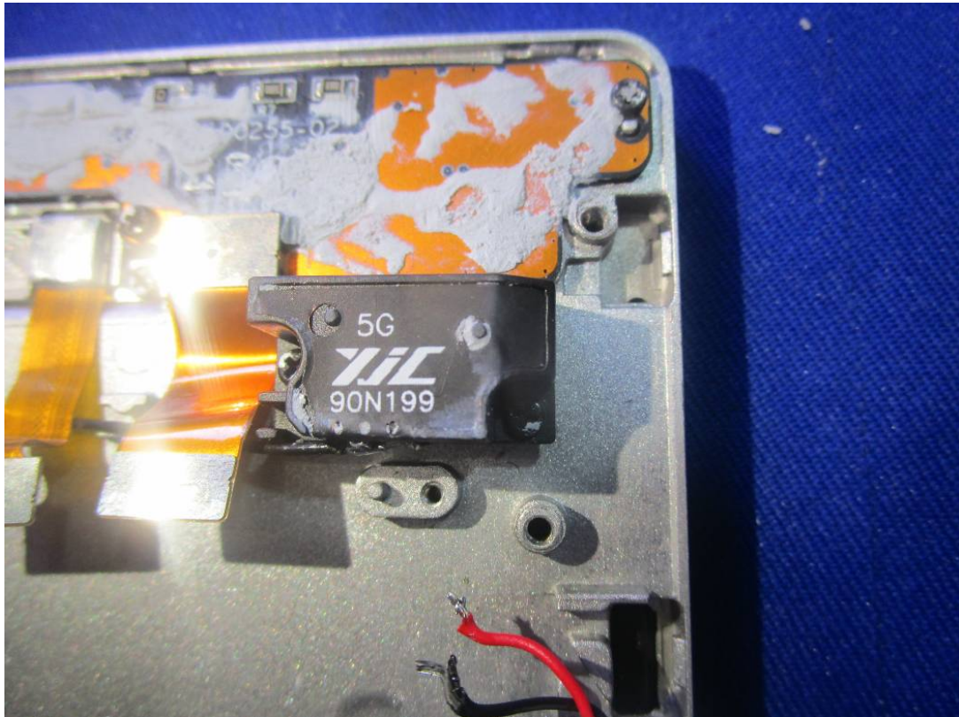
5G Antenna View
