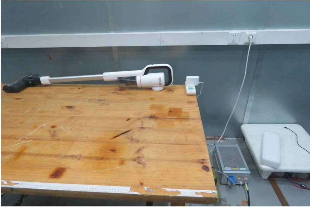
Picture 2 Conducted Emission Test Setup
