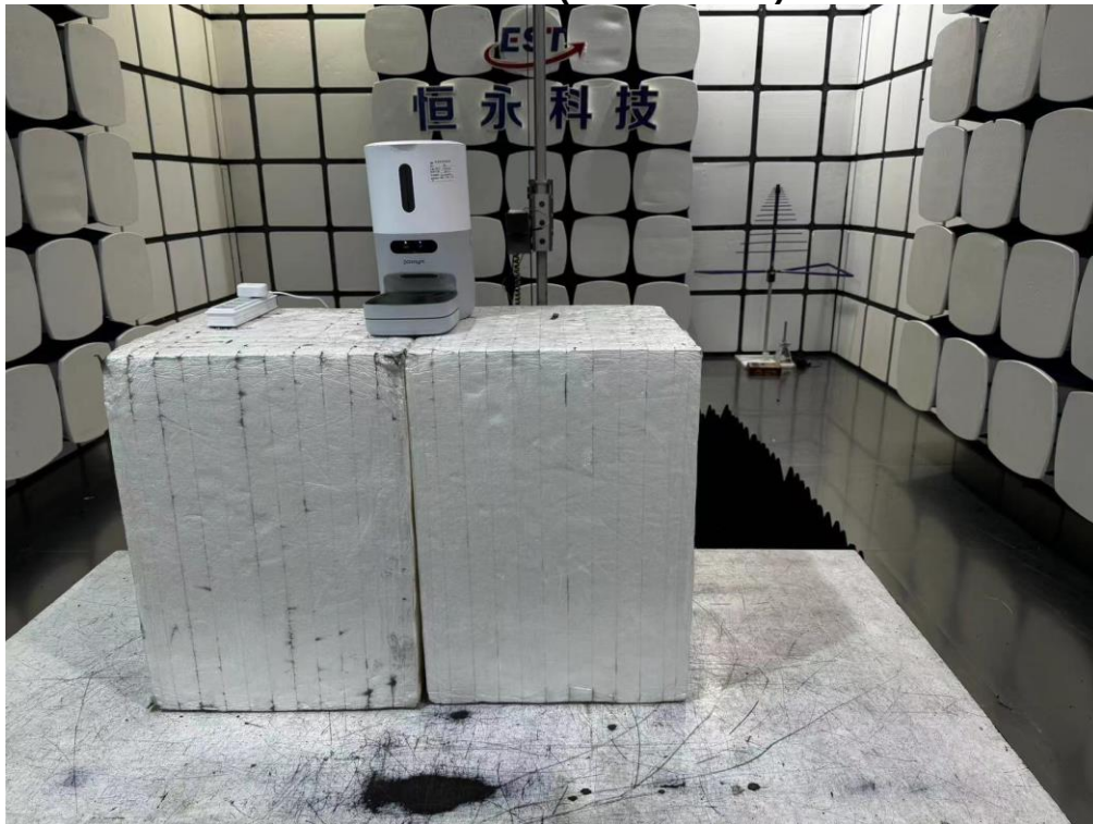
Radiated Test (Above 1GHz)
