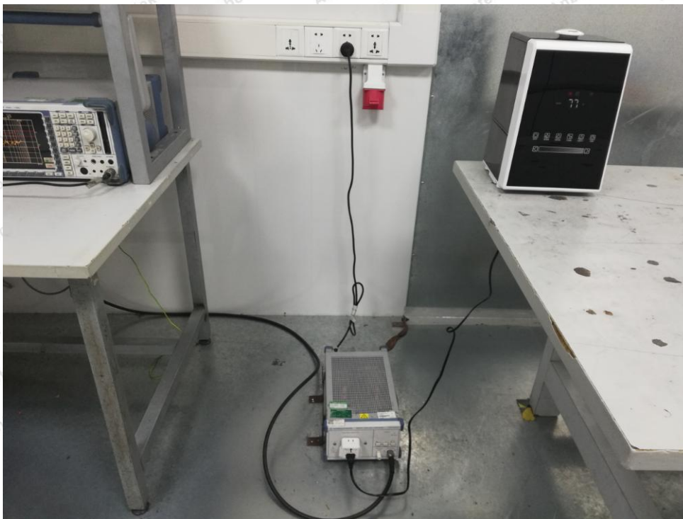
Photo of Power Line Conducted Emission Test
