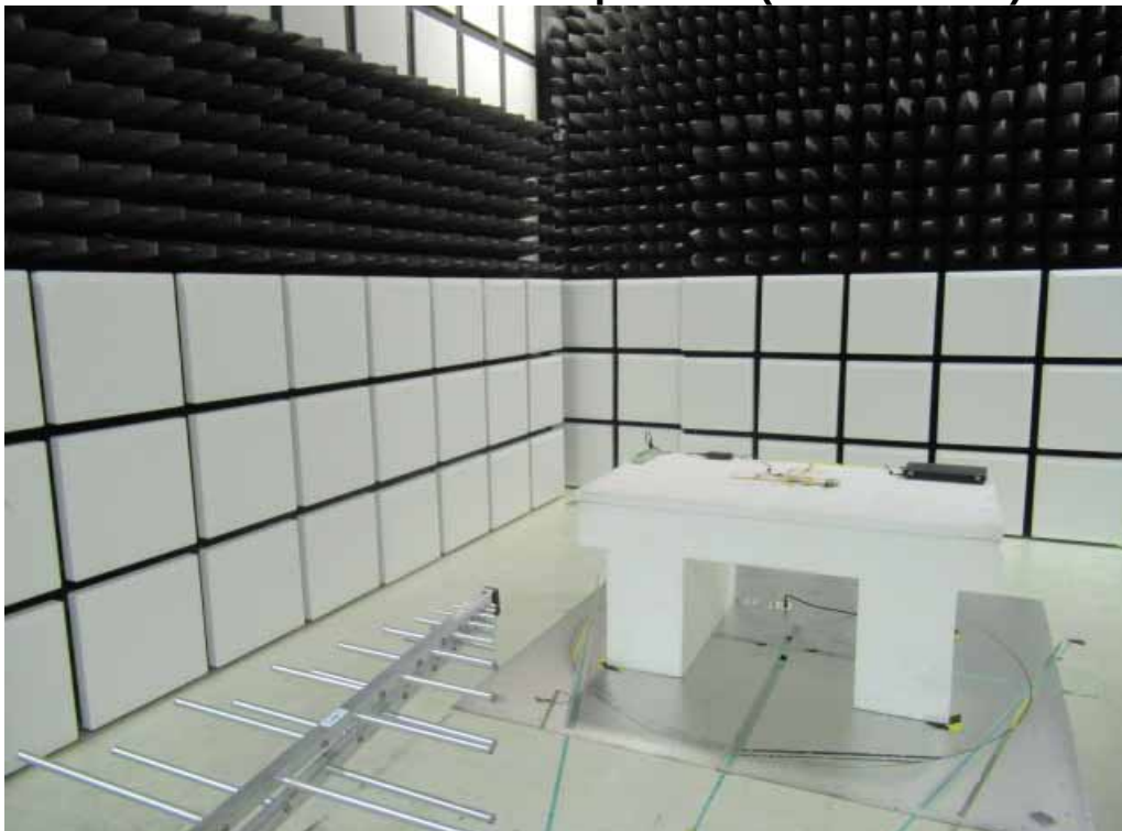
Radiated Emission Set up Photo (Below 1GHz)
