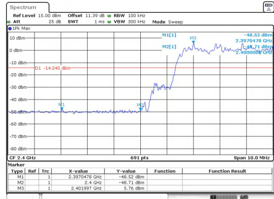
Out Of Band Emission(Left) \pi/4 DQPSK_2-DH5_Channel Hopping
