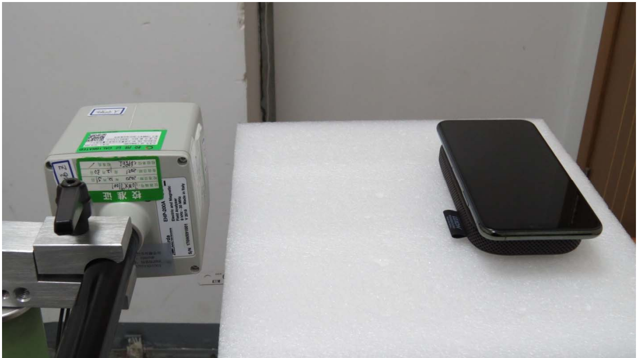
Picture 4: Right Side, the distance from EUT to the bottom of the Phantom is 15cm
