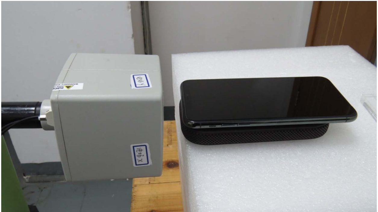
Picture 11: Top Side, the distance from EUT to the bottom of the Phantom is 15mm
