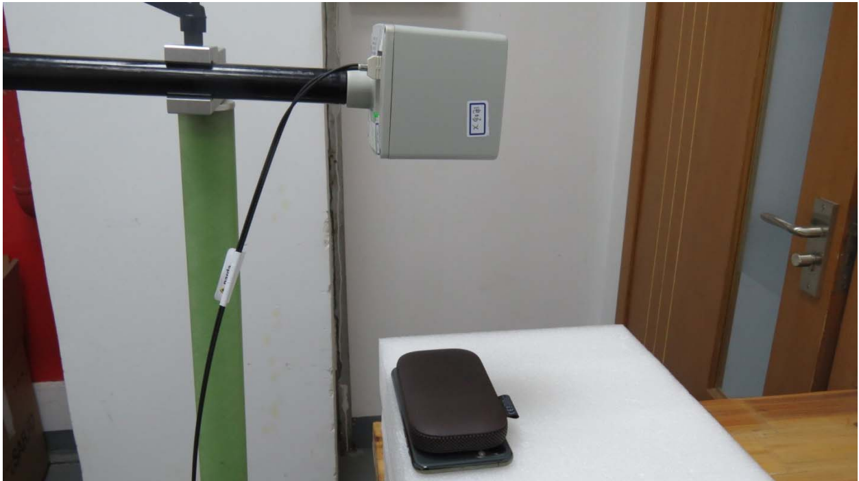
Picture 1: Back Side, the distance from EUT to the bottom of the Phantom is 20cm
