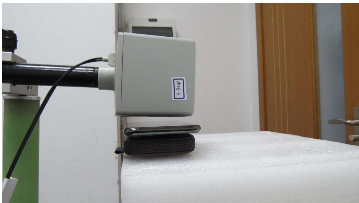
Picture 8: Front Side, the distance from EUT to the bottom of the Phantom is 15mm
