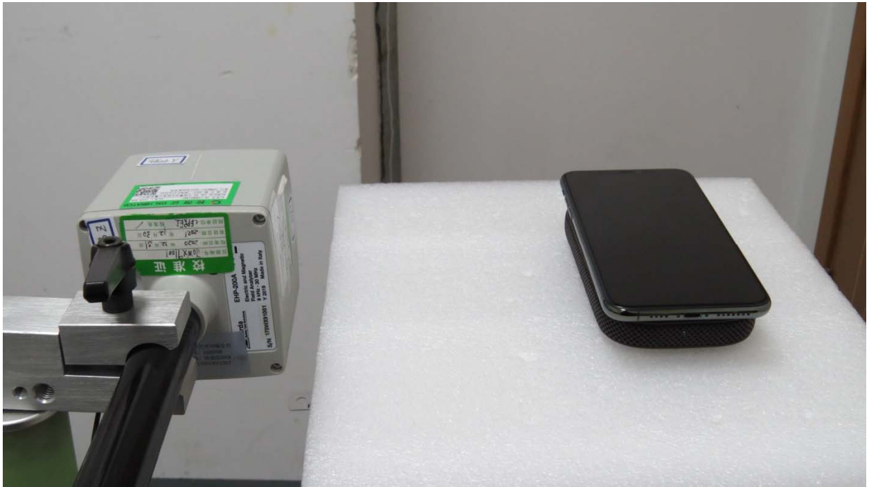
Picture 3: Left Side, the distance from EUT to the bottom of the Phantom is 15cm
