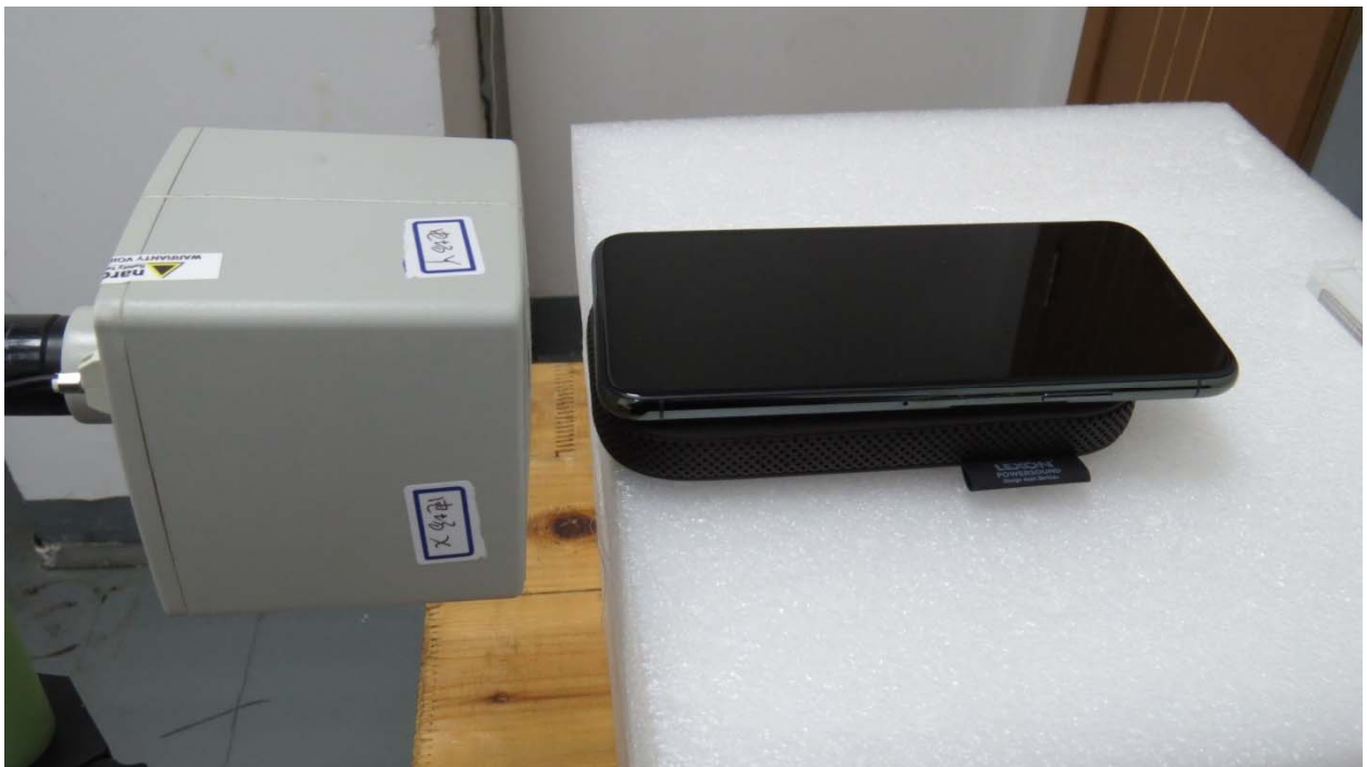
Picture 12: Bottom Edge, the distance from EUT to the bottom of the Phantom is 15mm
