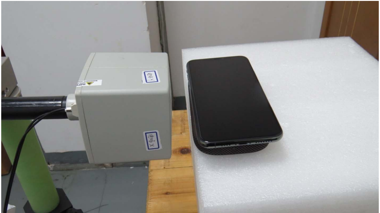
Picture 9: Left Side, the distance from EUT to the bottom of the Phantom is 15mm
