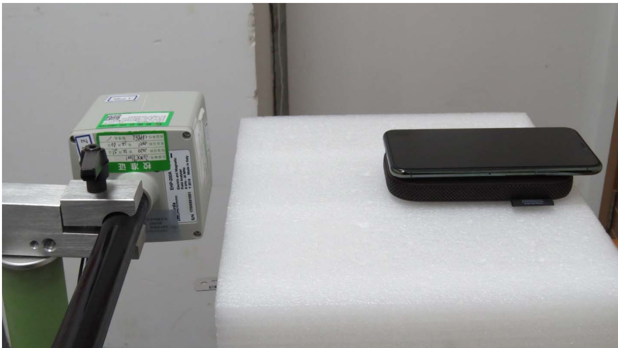
Picture 6: Bottom Edge, the distance from EUT to the bottom of the Phantom is 15cm
