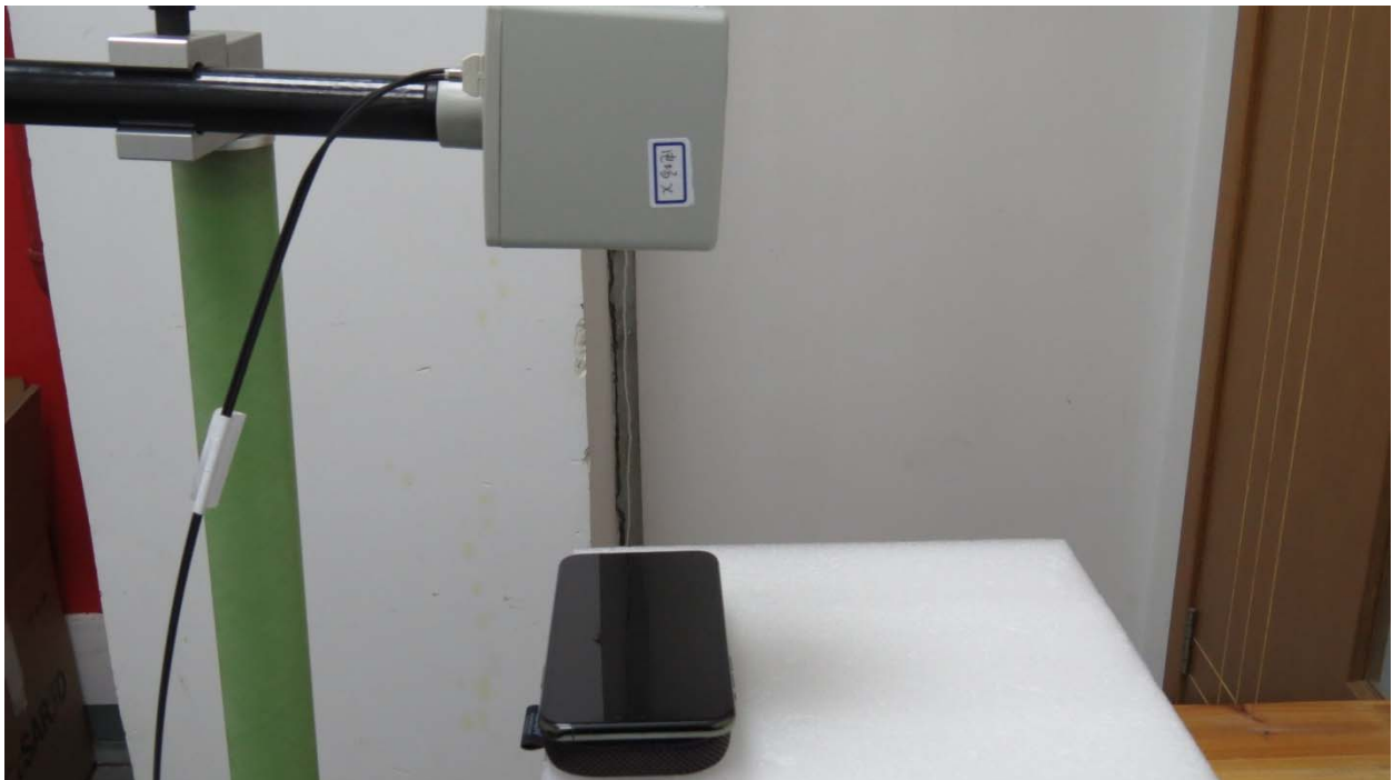
Picture 2: Front Side, the distance from EUT to the bottom of the Phantom is 20cm
