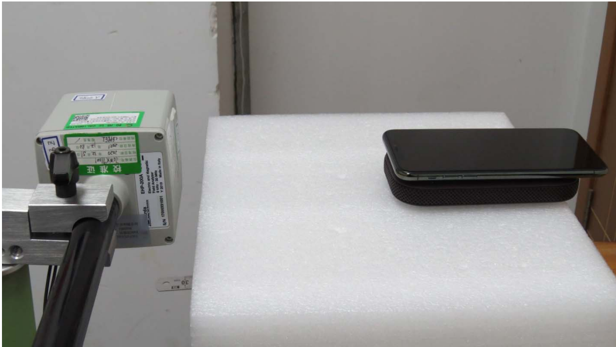
Picture 5: Top Side, the distance from EUT to the bottom of the Phantom is 15cm
