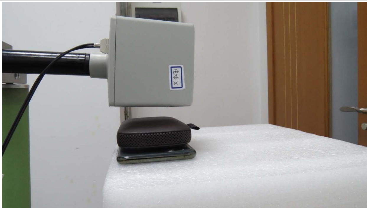
Picture 7: Back Side, the distance from EUT to the bottom of the Phantom is 15mm
