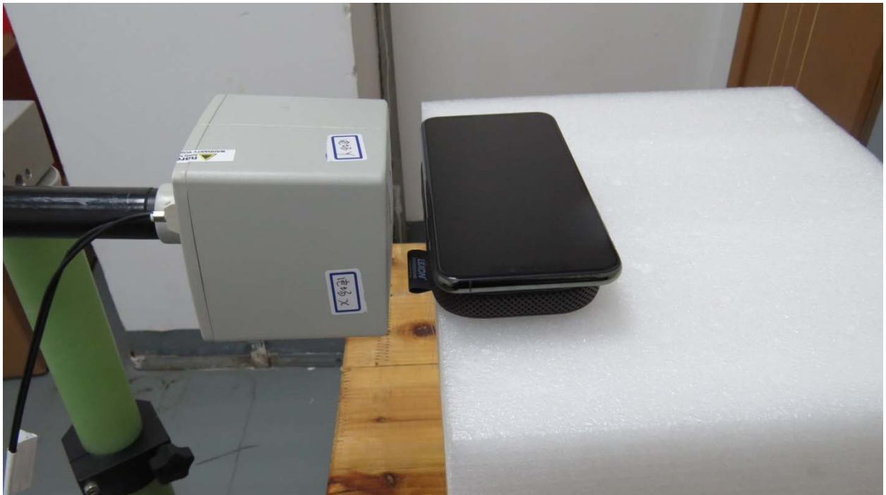
Picture 10: Right Side, the distance from EUT to the bottom of the Phantom is 15mm
