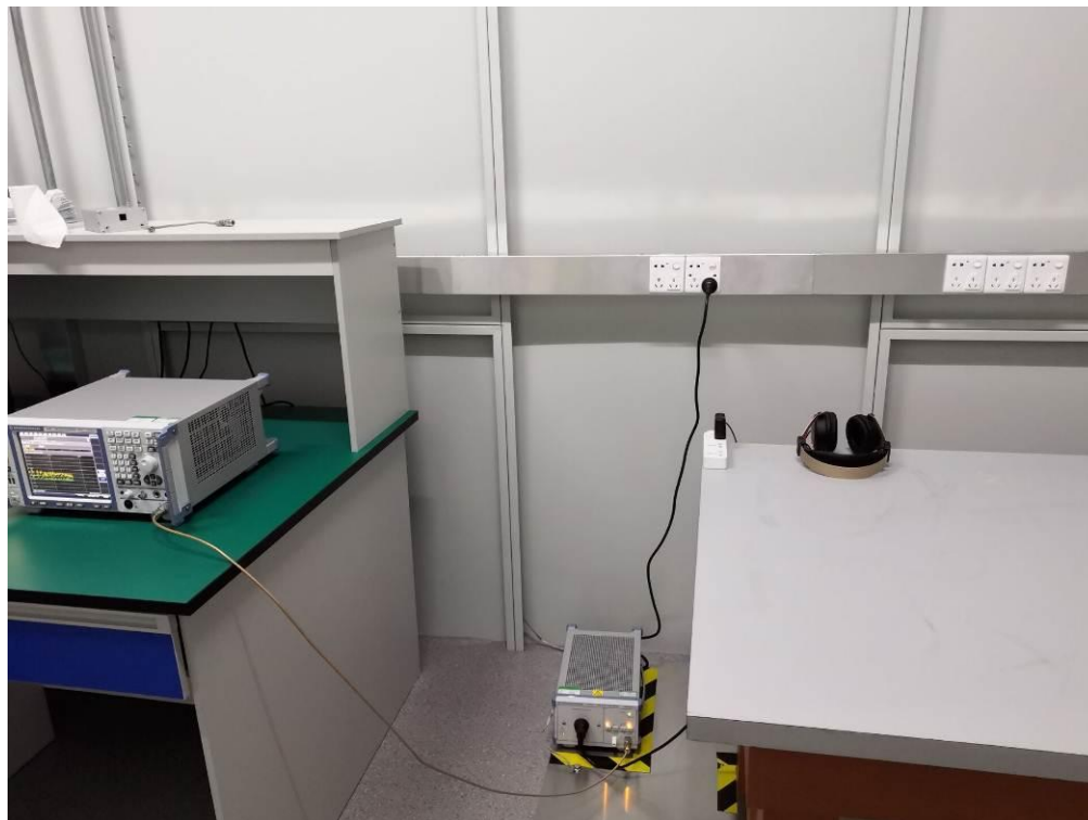
FCC RADIATED EMISSION TEST SETUP
