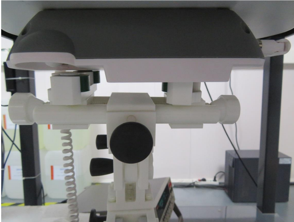
0mm body-worn Horizontal-Down Side Setup Photo(180° )
