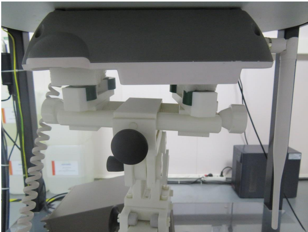
0mm body-worn Vertical-Bottom Side Setup Photo(90° )
