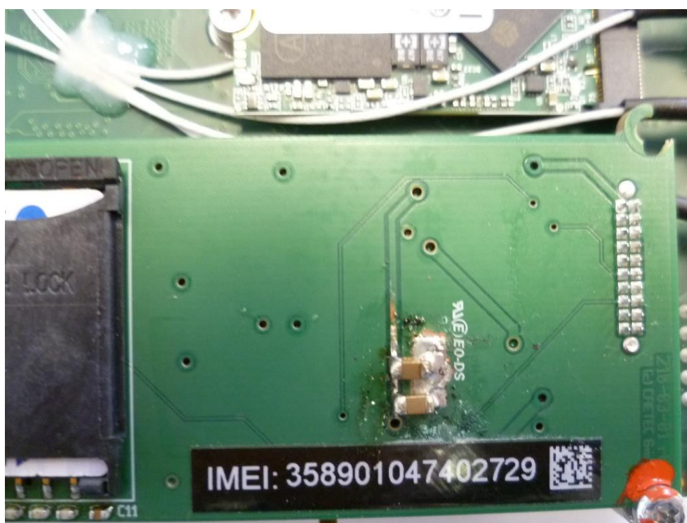
Figure 9: EUT modification to pass EMI AC
