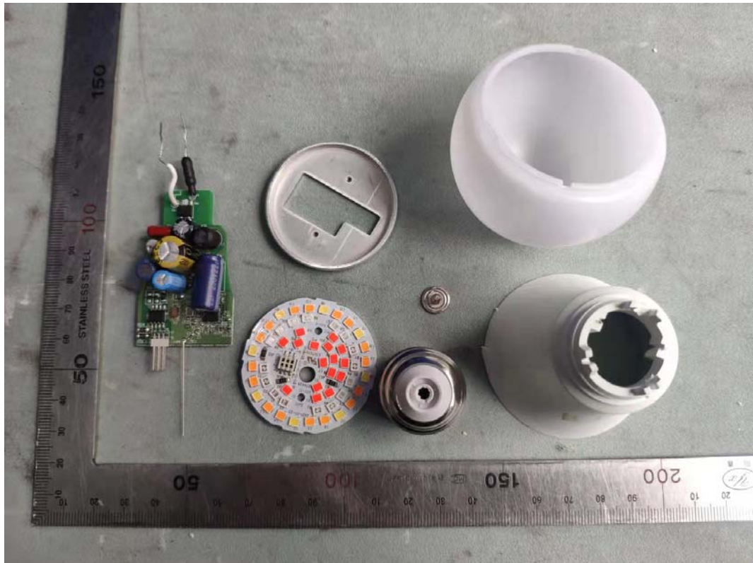
FIGURE 1 ABODE COLOR BULB (M/N: 104062/A) GENERAL APPEARANCE (COVER REMOVED)
