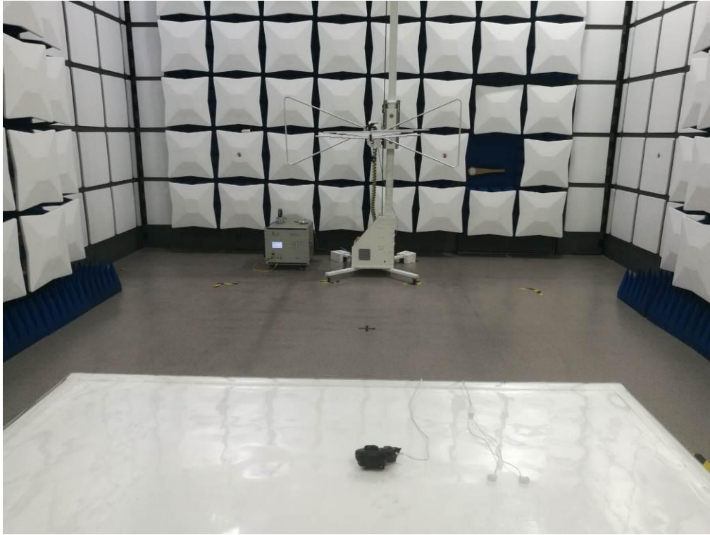
FCC RADIATED EMISSION TEST SETUP
