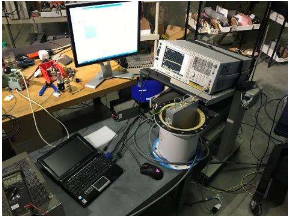
S-Band Conducted Antenna Port Measurements
