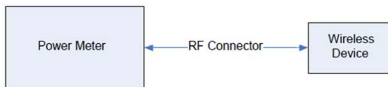
Figure 8.1.1 Power Measurement Setup
