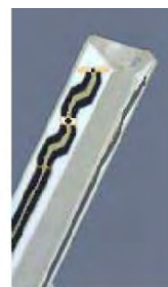
Figure E.2.2 Probe Thick-Film Technique
