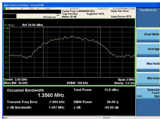
20dB Bandwidth plot on channel 78 (3Mbps)
