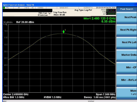
Peak output Power plot on channel 78 (2Mbps)
