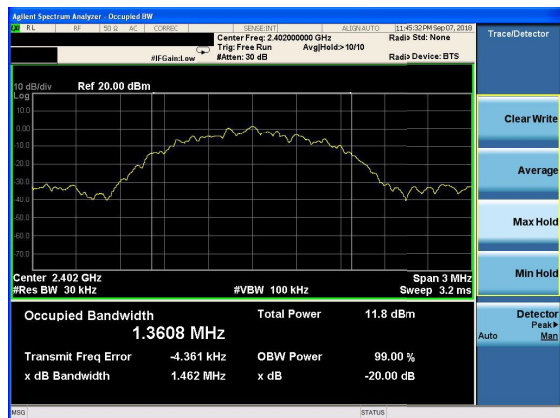
20dB Bandwidth plot on channel 39 (3Mbps)
