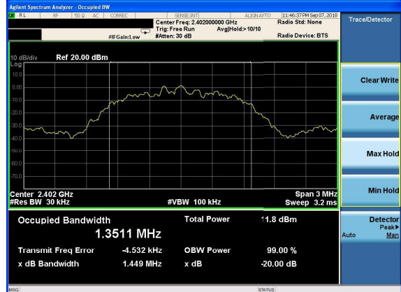
20dB Bandwidth plot on channel 39 (2Mbps)
