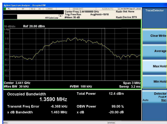
20dB Bandwidth plot on channel 78 (3Mbps)
