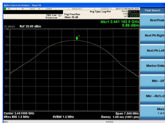
Peak output Power plot on channel 39 (2Mbps)
