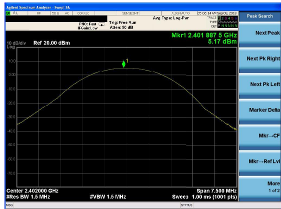
Peak output Power plot on channel 39 (2Mbps)
