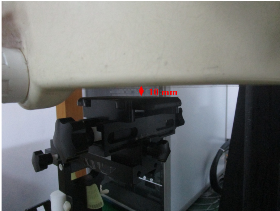
Body (Worn) Front Setup Photo (10mm)
