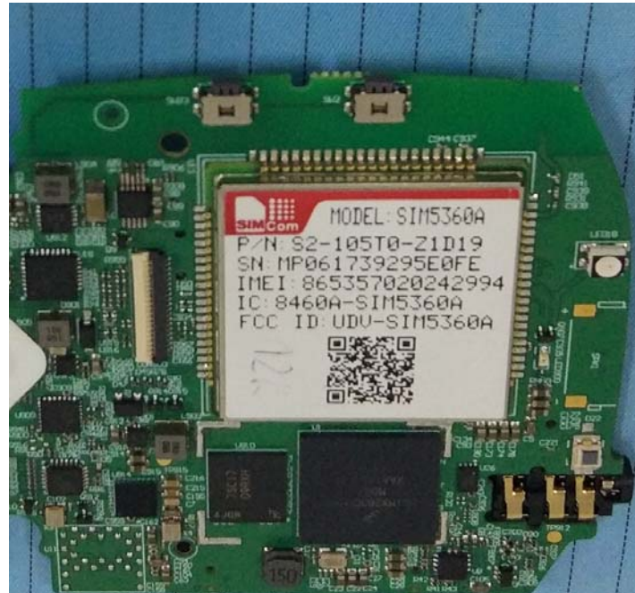
EUT – RF Module View
