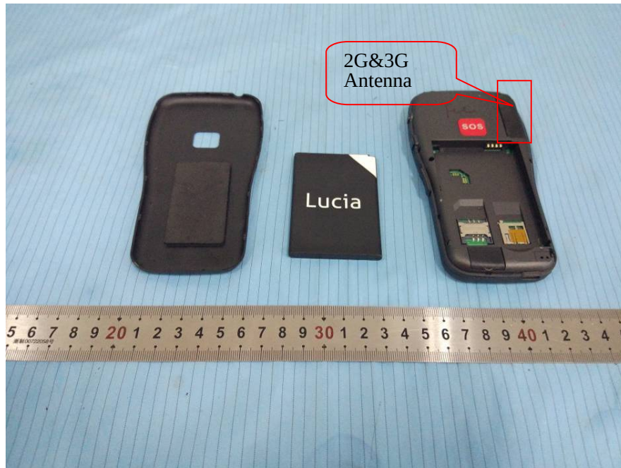
EUT – Cover off View 1
