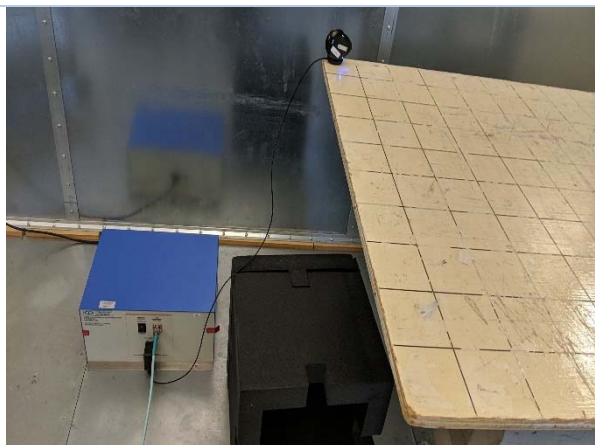
Conducted Emissions (Right Unit)
