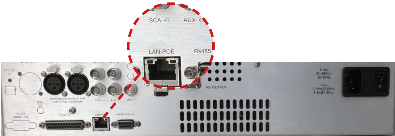
Fig. C1: Zoom of the LAN-POE connector on rear view of the transmitter
